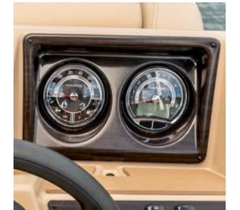
INTEGRATED DEPTH SOUNDER ON STANDARD GAUGES
