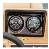
INTEGRATED DEPTH SOUNDER ON STANDARD GAUGES
