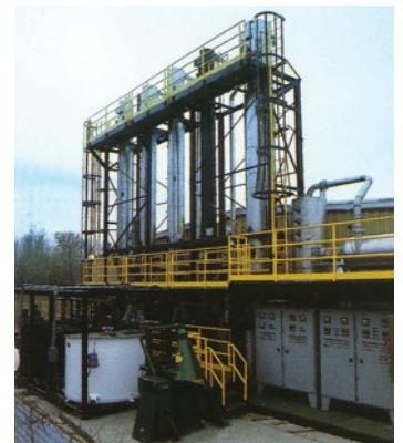
Tri-NO x Multi-Stage Multi-Chem system with acid recovery.
