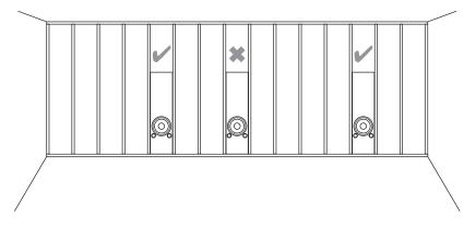
In some situations, it may not be possible to install the subwoofer into a wall. In this case the ceiling, floor, or even a closet are options. Wherever the AMC Sub 10 is installed it must be securely mounted. If it is not securely mounted, its substantial bass output may produce rattles. In addition, be sure that the connectors are accessible for electrical hook-up.
