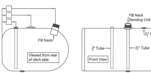
Please note: All sizes are NPTF unless otherwise noted and reference all measurements from the lateral weld seam and the end cap weld seam to the center of the fittings.
