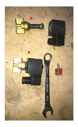
In most cases when a solenoid goes bad what happens is the ignitor buzzes (sparks) trying to ignite burner but no gas is coming through the line and therefore you see no movement on the gas gauge and there is no gas getting to burners to ignite.
