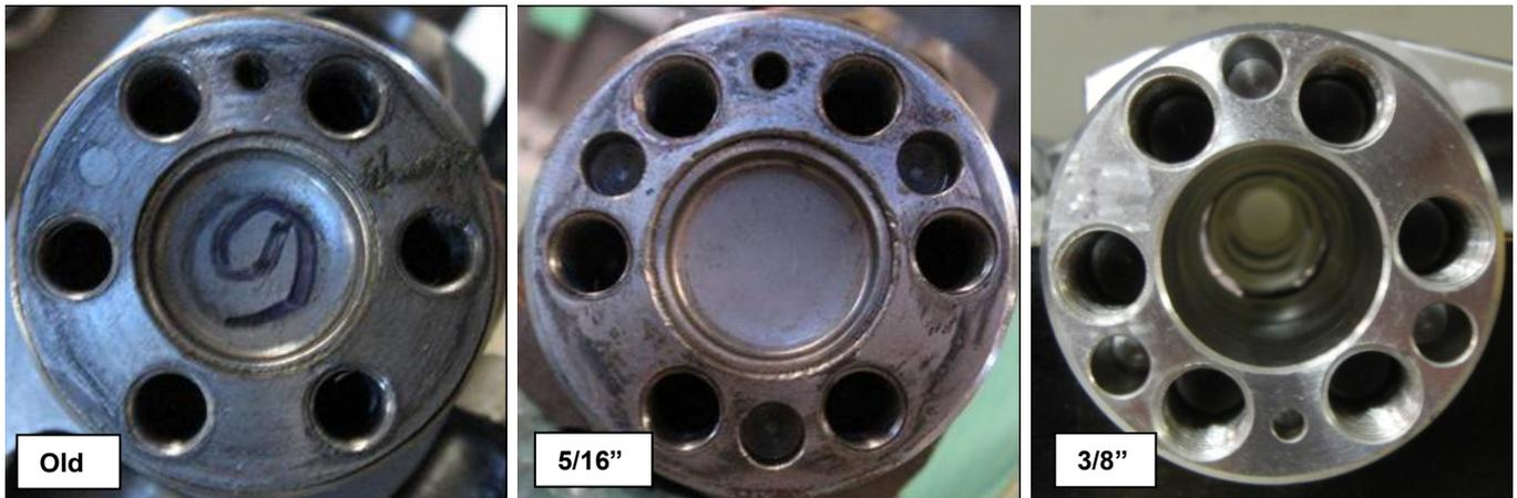
Figure 64 – Crankshaft End Detail (Dowel Holes)
