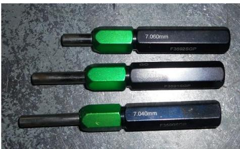
Go-Nogo gauges are used to quickly and accurately check the inner size of a valve guide. Sizes 7.03 / 7.04 / 7.05 / 7.06 / 7.07 / 7.08. Gauges produced by 'Prittie' ([www.prittie.com.au](http://www.prittie.com.au)) are used in the factory.
