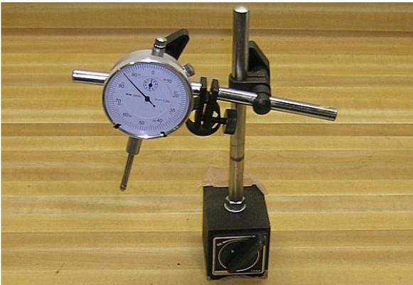
As well as Crankshaft run-in, a dial gauge is also used to locate top dead centre (TDC) in the cylinder.
