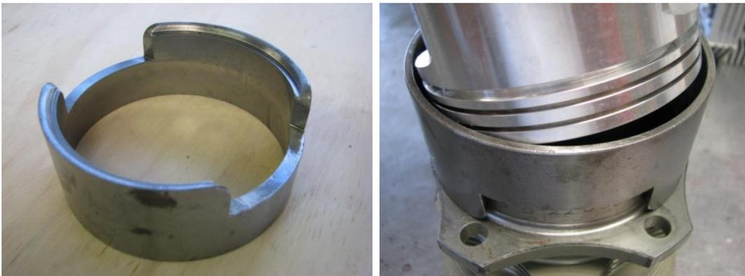
Figure 18 – Piston & Ring Installer
