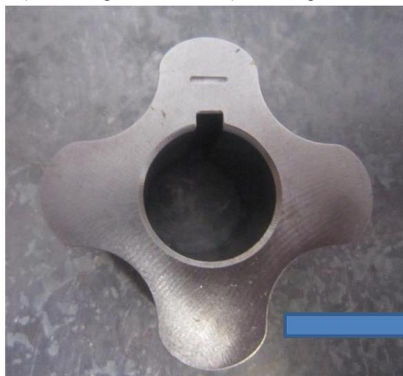
**Figure 82: Broad lobe inner gear with line marking.**
