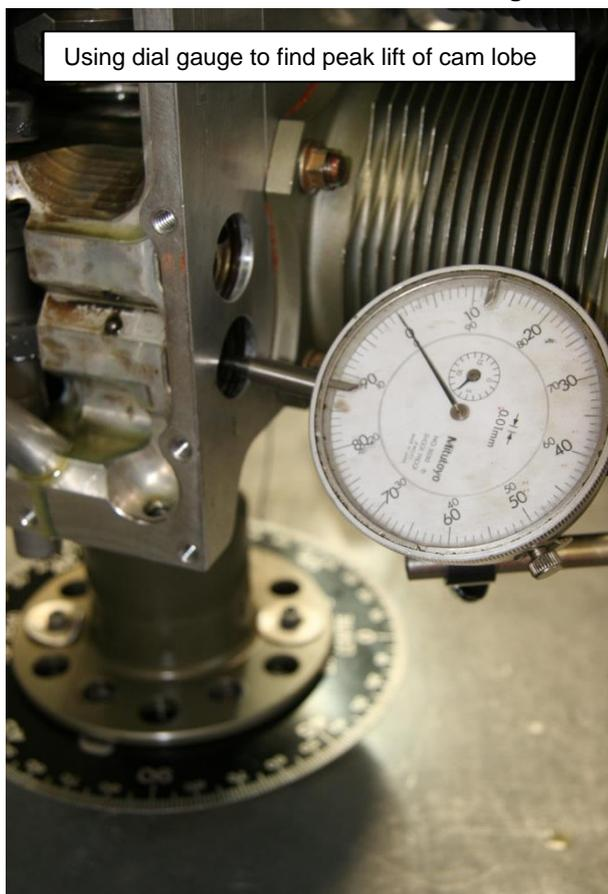
Extremes of engine rotation for 0.5mm drop on dial gauge – peak lift is halfway between these points
