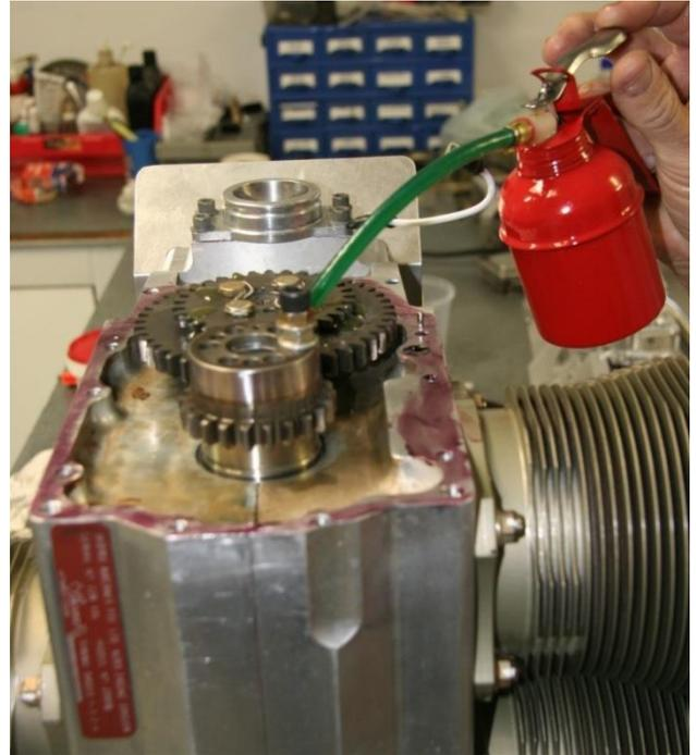
Figure 172 – Sealing Engine Mount Plate
