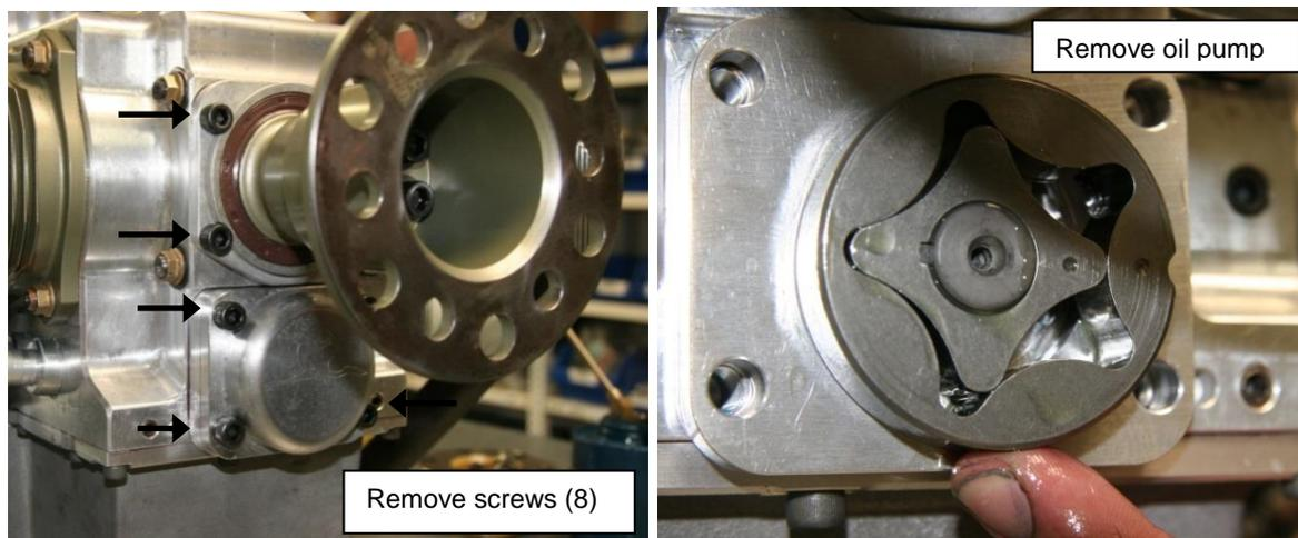
Figure 56 – Front Seal & Oil Pump Removal
