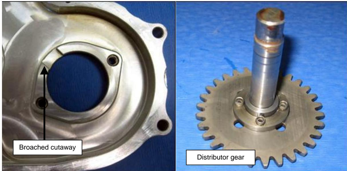
Figure 109 – Distributor Gears & Case
