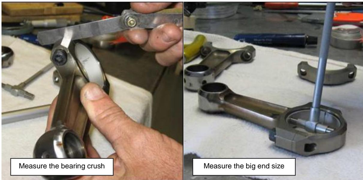
Measure the bearing crush
