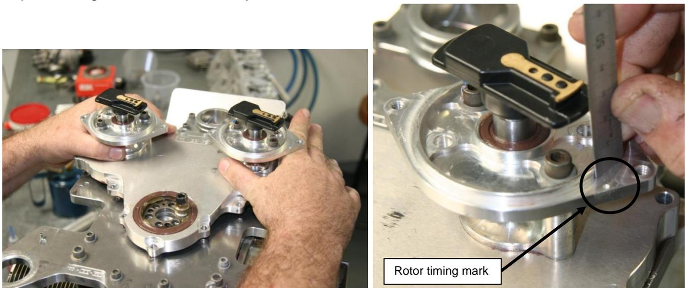
Figure 176 – Setting Distributors, Checking Rotor Position
