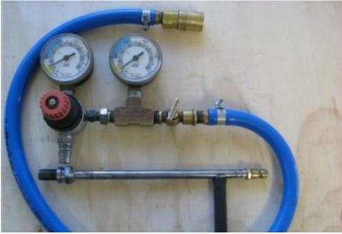
An adaptor is made by welding a compressor air fitting to the base of an old spark plug. The adaptor is screwed into the spark plug hole of a head and connected to the leak-down tester to check the condition of the cylinder assembly.
