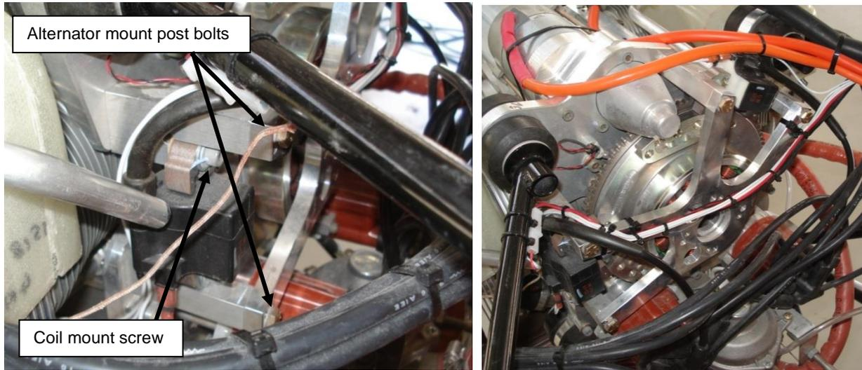
Figure 184 – Ignition Post & Alternator Stator Installation
