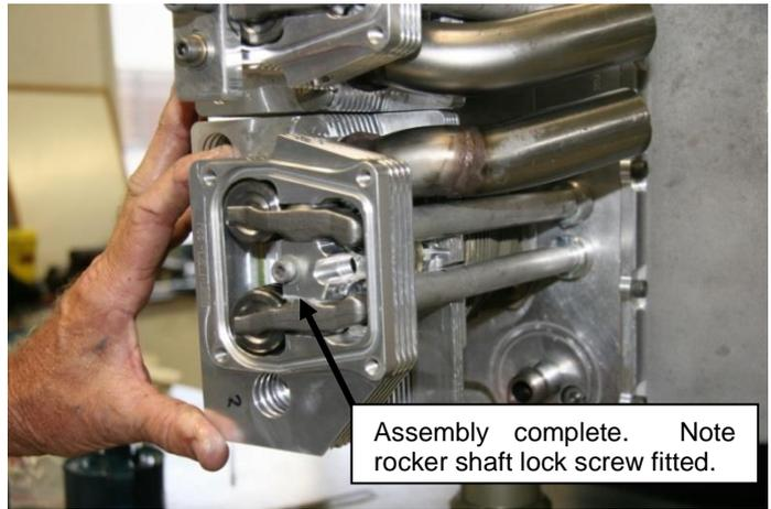
Figure 192 – Fitting Rockers #3
