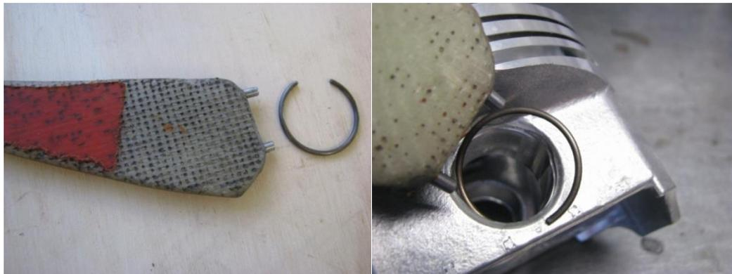
**Figure 134 – Fitting Wire-Type Piston Circlips**
