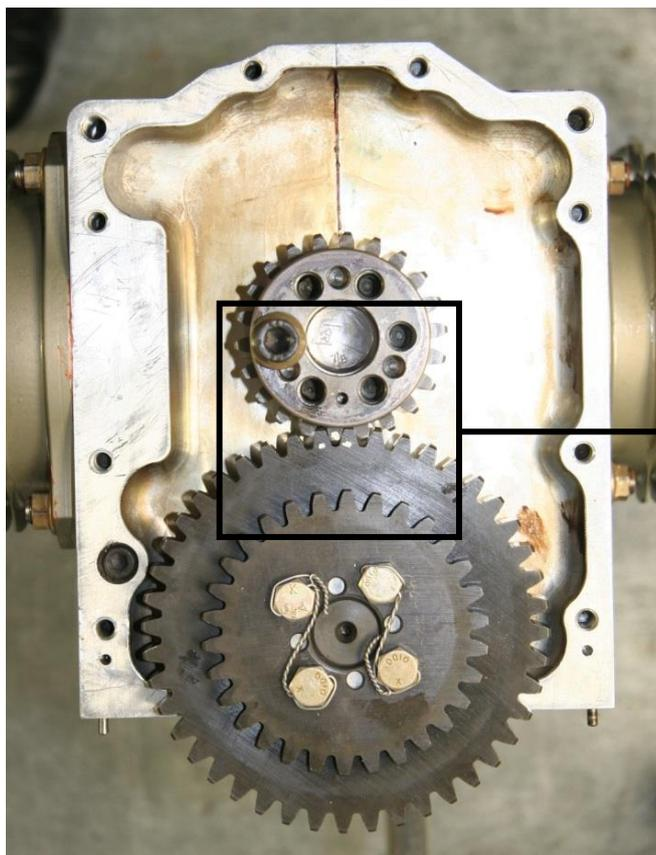
Datum hole aligned with timing marks on gears.
