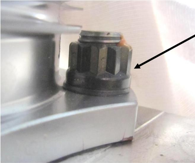
Nut on assembled engine. Note “new type” barrel, small-flange 12-point nut & washer shown.
