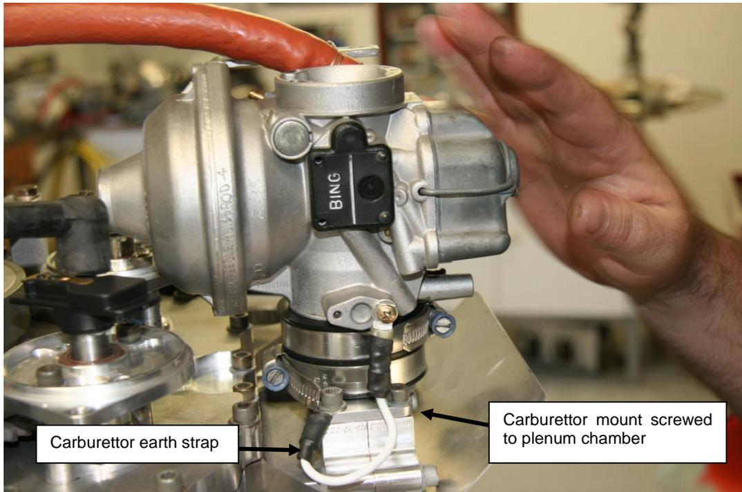
Figure 197 – Fitting Carburettor
