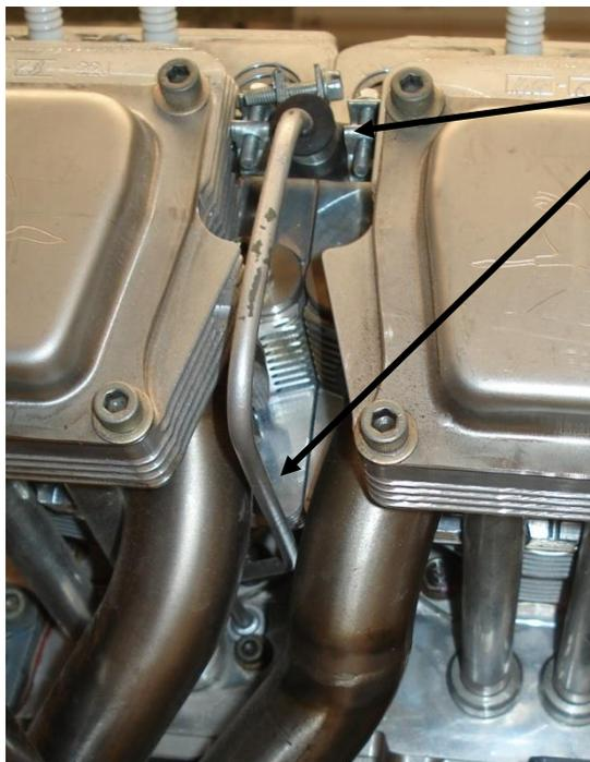
Oil feed tube from crankcase port to cylinder heads
