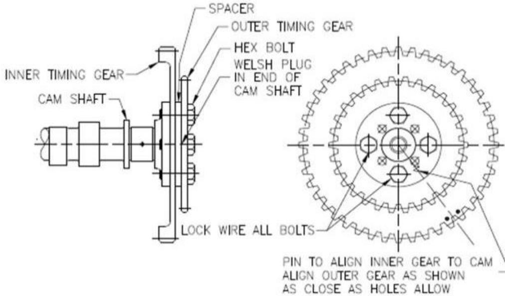
Figure 129 – Cam Timing Gear Assembly
