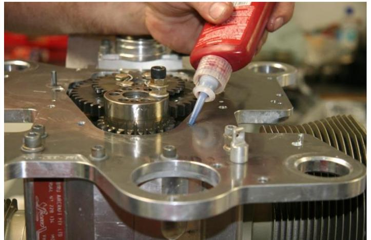
Figure 173 – Fitting Engine Mount Plate
