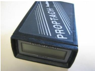
An accurate optical tachometer. Reads directly from reflective strips fitted to the propeller and is used whenever an accurate check of RPM is required. Will usually read propeller RPM in sunlight without reflective strips.
