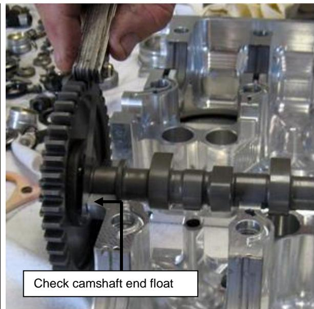
Figure 130 – Assembling Cam & Fitting to Crankcase
