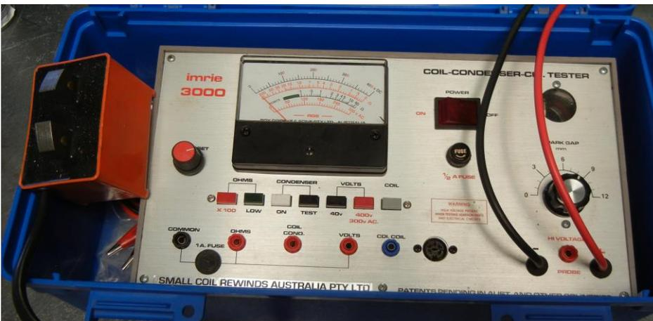
Used to test ignition coil performance.
