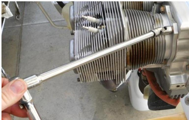
**Figure 164 – Universal Joint tool FU14B (FU16B for 1/2" Socket)**
