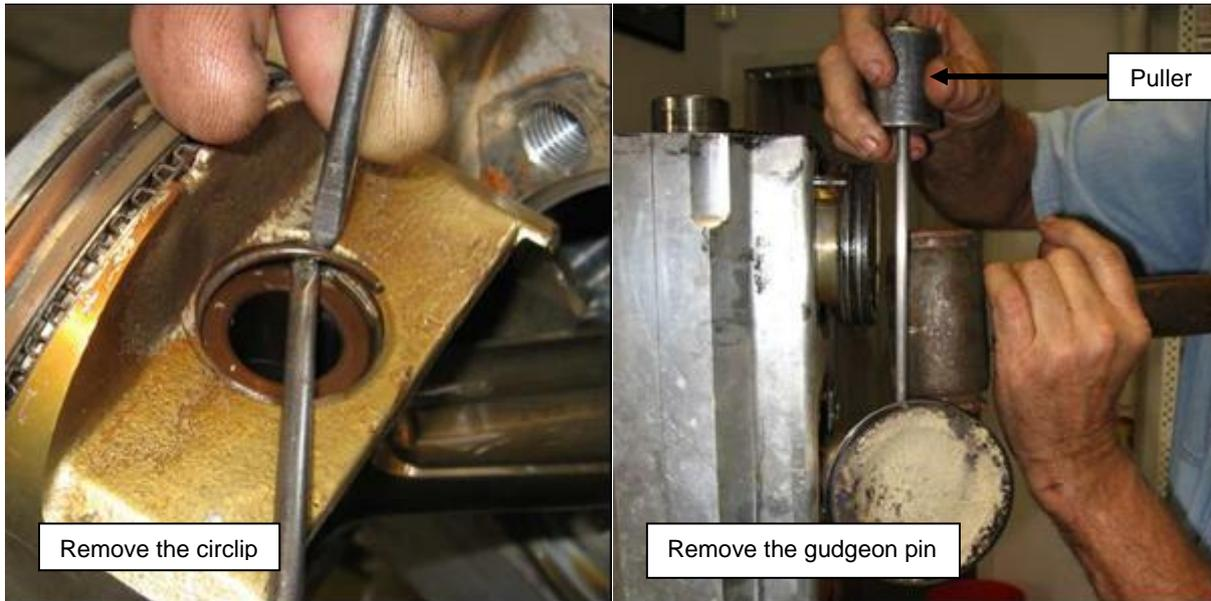
Figure 55 – Remove Pistons
