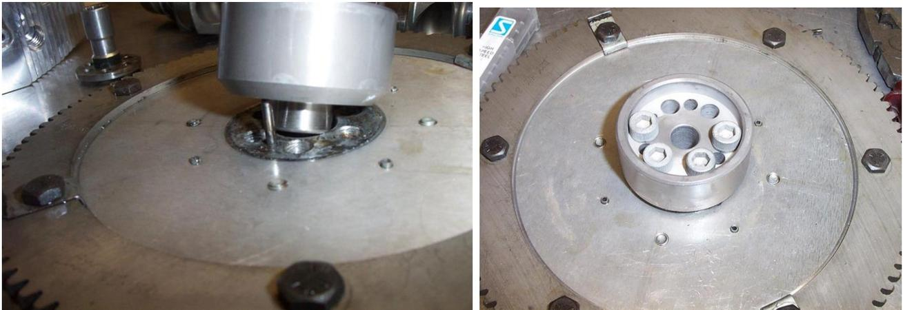
Figure 218 – Aligning Guide & Fitting To Flywheel.
