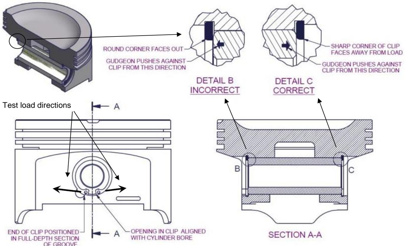
Figure 136 – Clip Installation Detail
