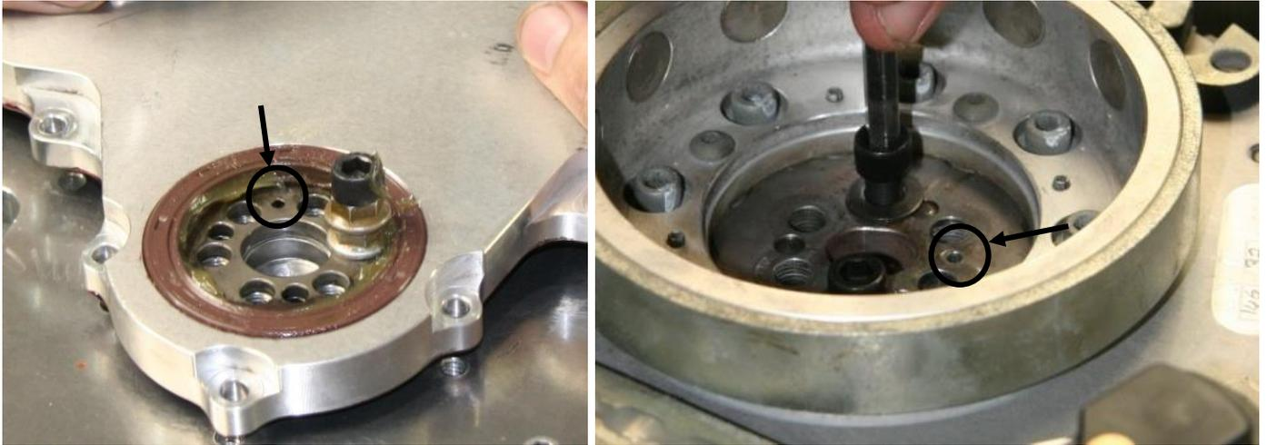
Figure 180 – Flywheel &amp; Crank Timing Marks
