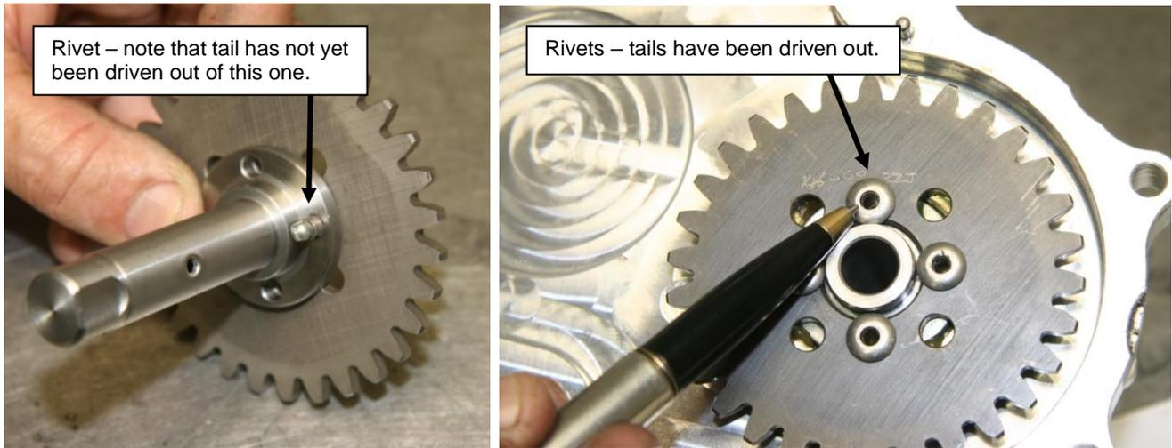
Figure 154 – Assembling Distributor Gear to shaft
