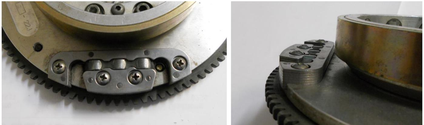
Figure 149 - Laminated Magnet retaining pole plates
