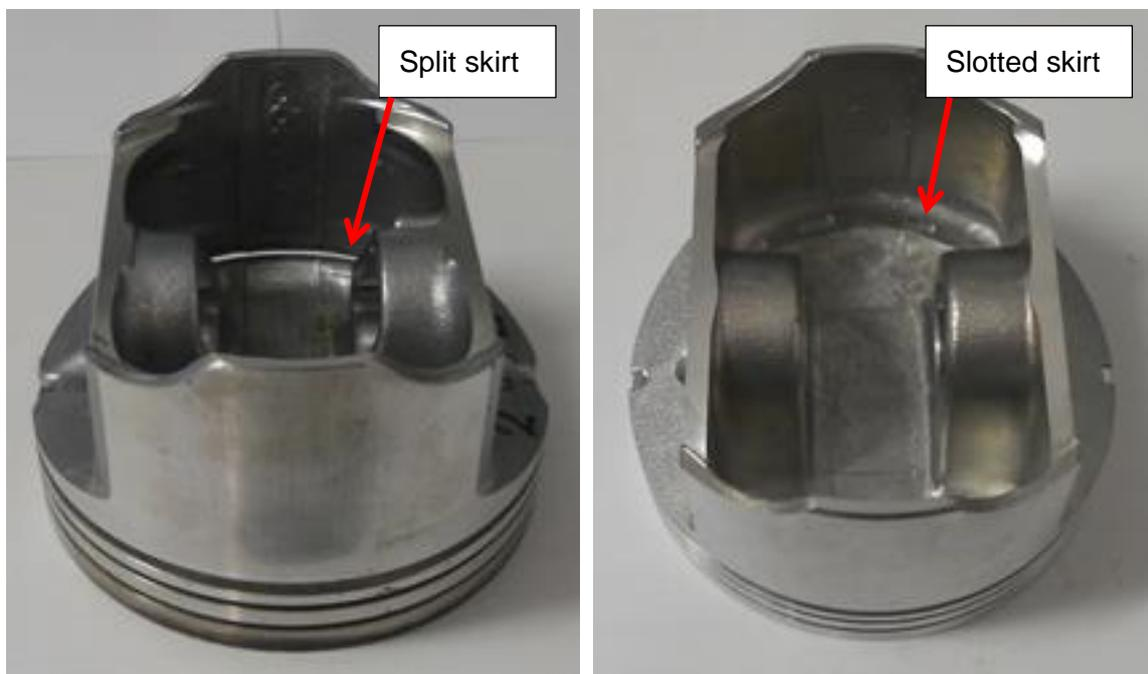
Figure 140 - Split and Slotted skirt pistons
