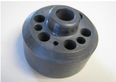
A tool which is used to drill dowel holes in early model crankshafts and flywheels. Jabiru Service Bulletin JSB012 refers.
