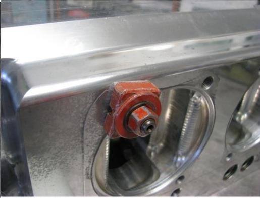
**Figure 32 – Crankcase Dry Fit Through-Bolts and Nuts**
