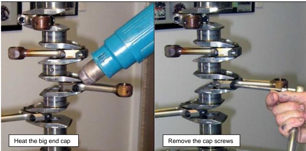
Figure 61 – Remove Con-Rods
