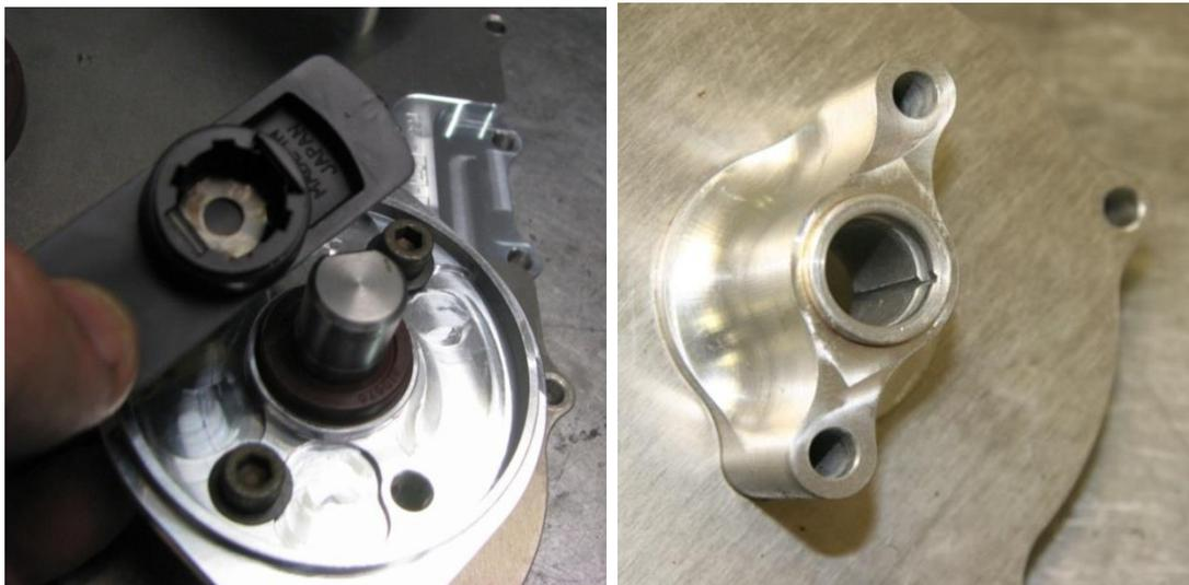
Figure 153 – New Distributor Shaft Bush Fitted – nopic x 1
