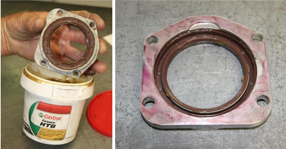
Figure 202 – Front Seal Housing Ready To Fit
