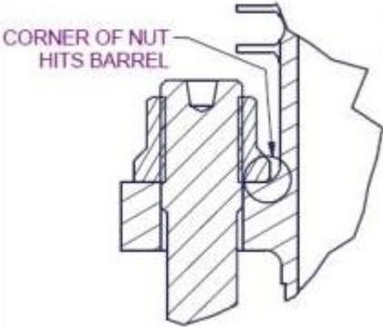
**Figure 142 – Through Bolt Nut Installation Detail**
