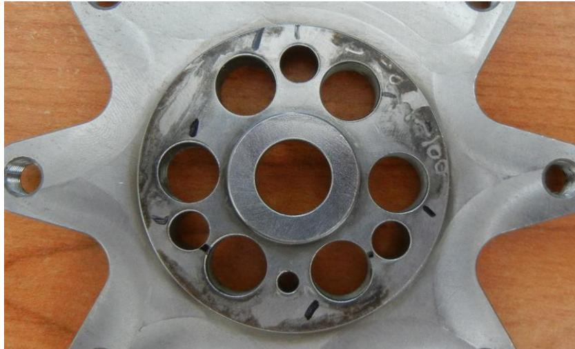
**Figure 104 – Damaged Flywheel “Starfish”**
