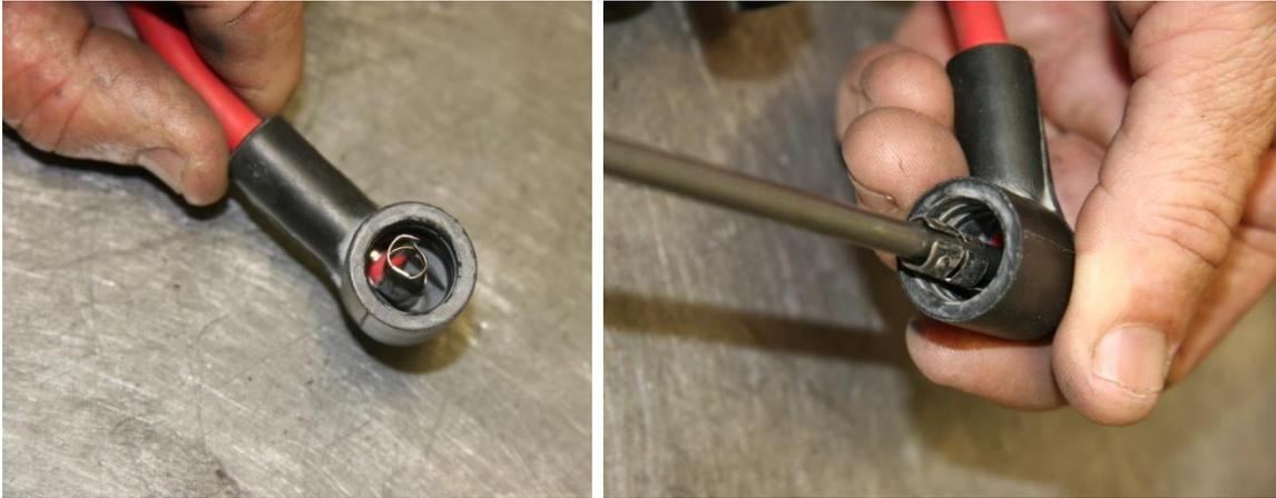
Figure 110 – Adjusting High Tension Lead Caps
