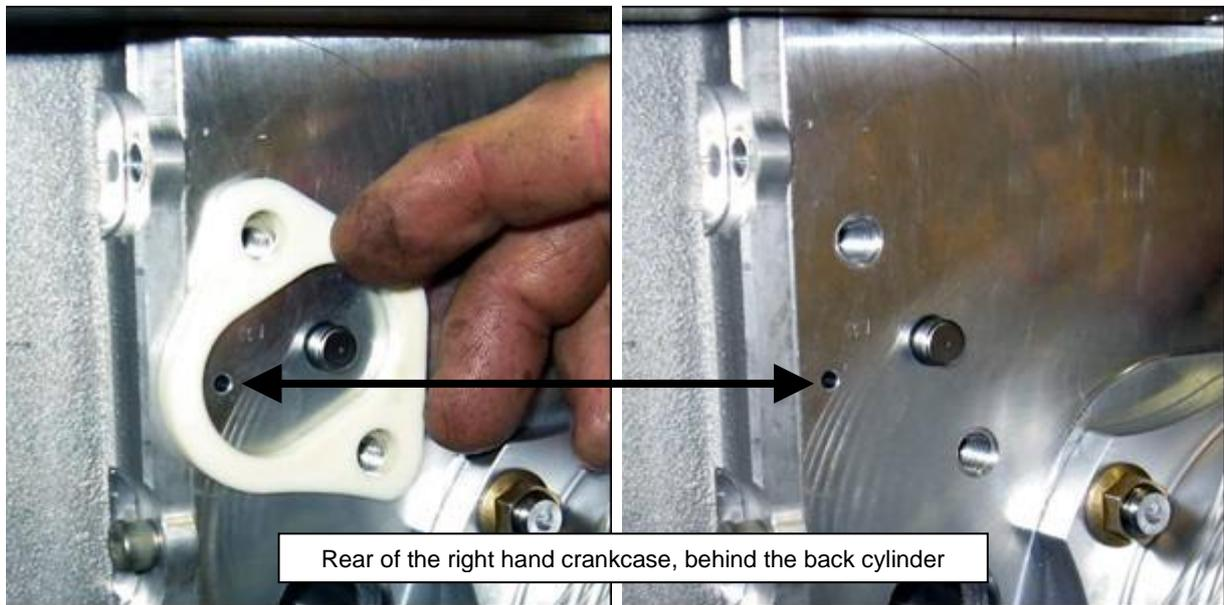
Figure 70 – Fuel Pump Oil Drain
