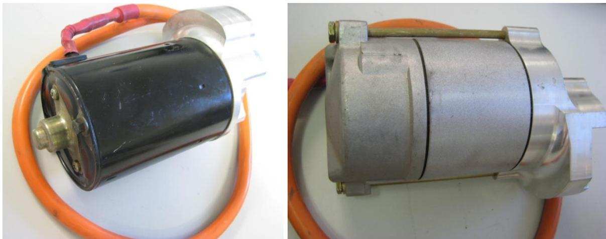
**Figure 105 – Starter Motor Old & New**
