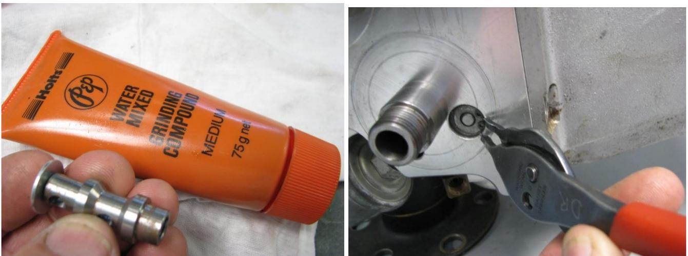
Figure 207 – Lapping Oil Pressure Relief Valve
