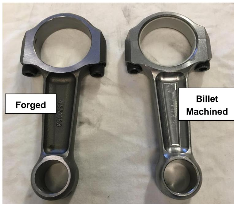
**Figure 122 - Forged conrods vs Billet machined conrods**
