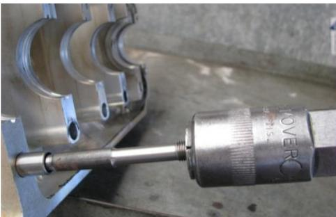
A tool which clamps onto the tip thread of the stud, holding it tightly and allowing the stud to be screwed out of the crankcase.
