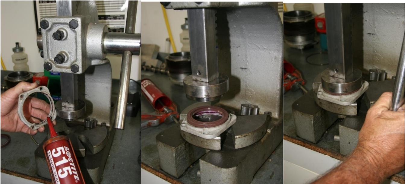
Figure 201 – Fitting Seal To Housing
