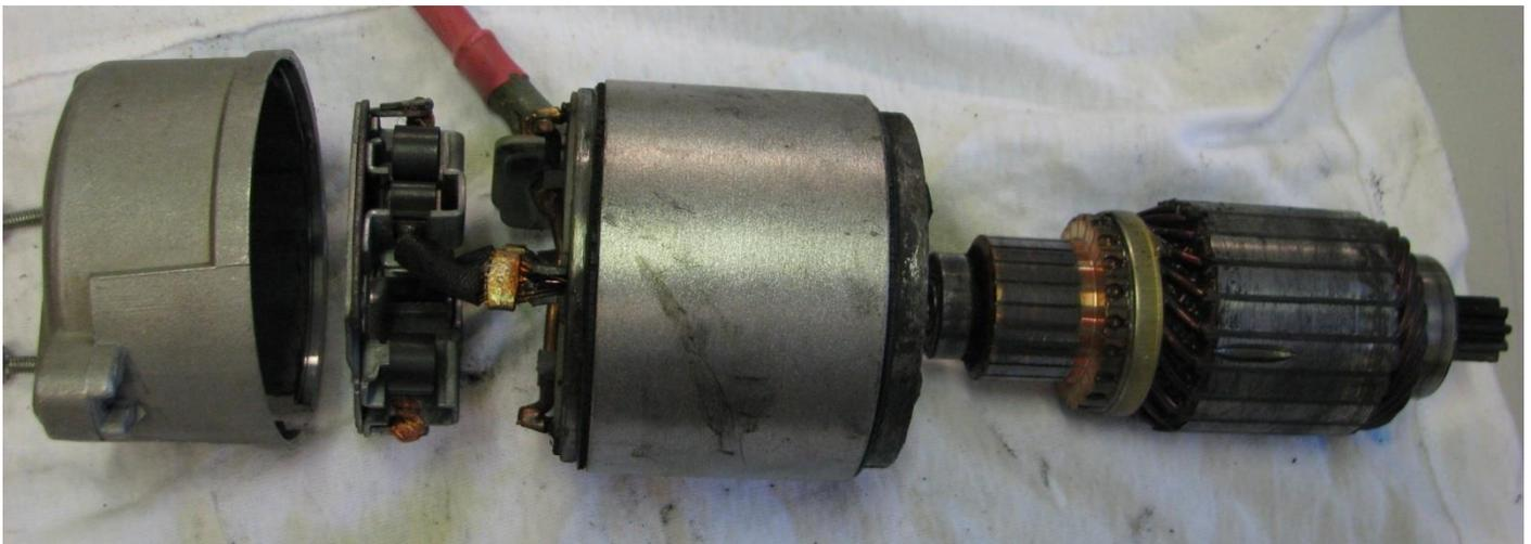
**Figure 106 – Typical Disassembled Starter Motor**
