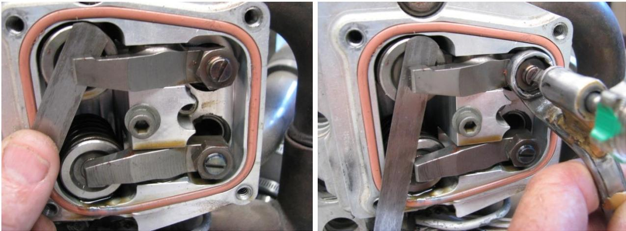
Figure 194 – Valve Clearance Adjustment (Solid Lifter)
