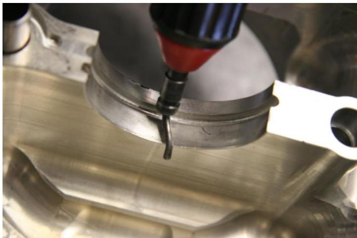
**Figure 213 – De-Burring Crankcase After Surfacing & Line Boring**
