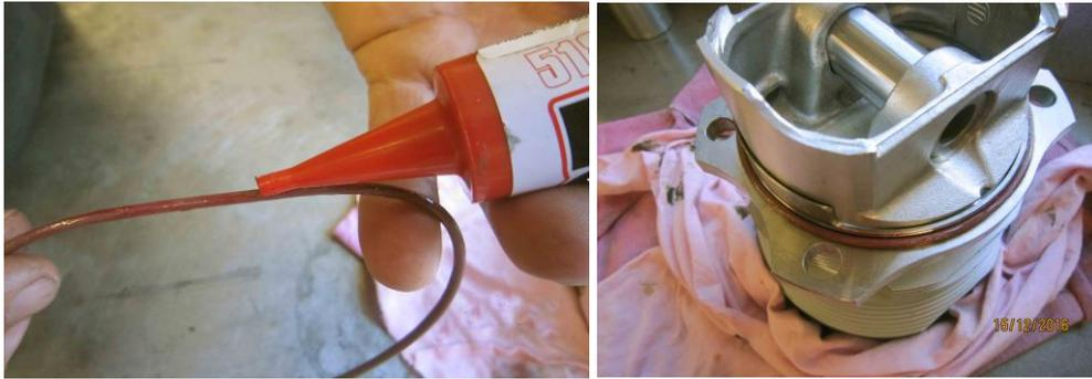
Figure 159 – Applying Sealant and O-Ring to Cylinder Base
