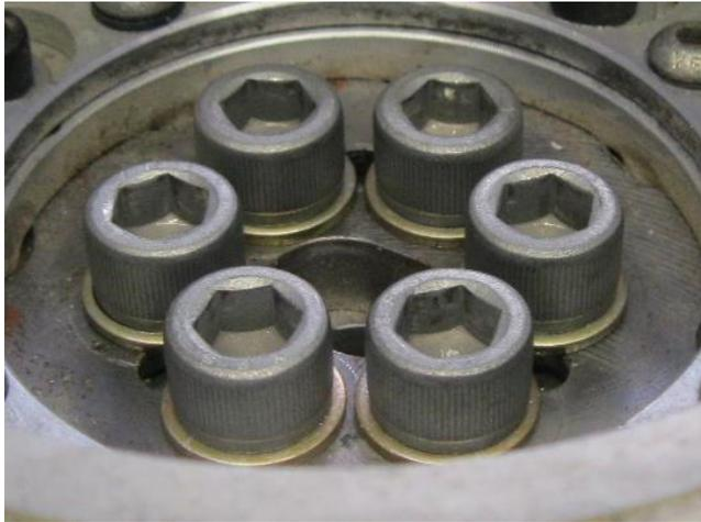
Install capscrews with 6 old plain washers to **15ft.lb** and then the **Prescribed Torque** (Table 9) progressively using diagonal pattern shown in Figure 181
