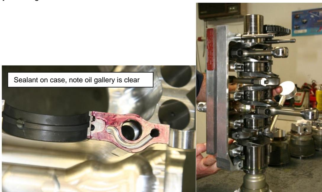
Figure 156 – Applying Sealant to Case, Fitting to Crank
