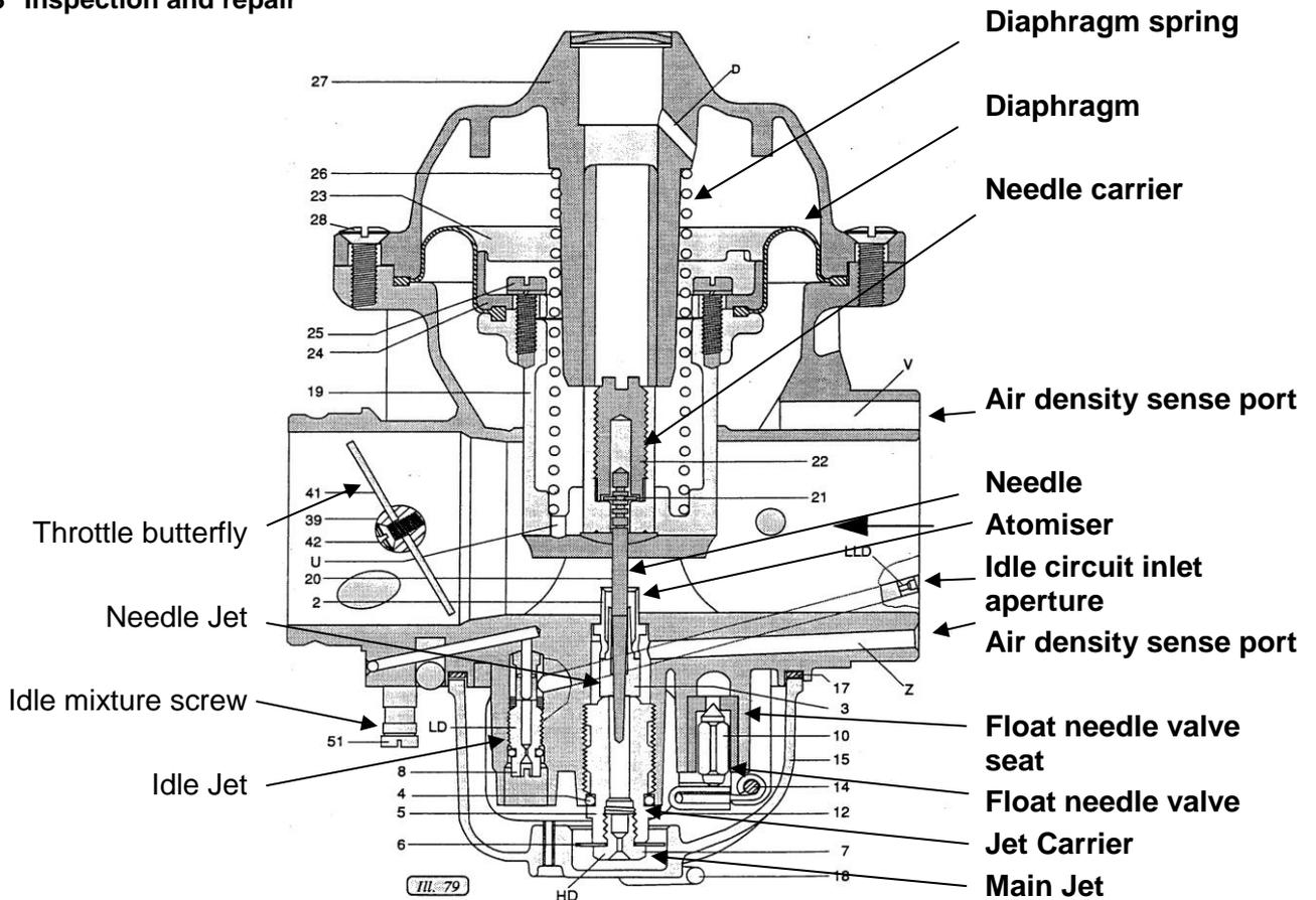
Figure 112 – Carburettor Schematic
