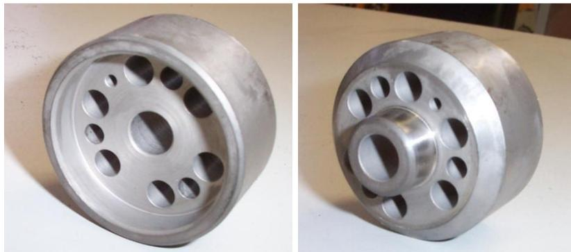
Figure 214 – Drilling Fixture – Crankshaft Side on Left, Flywheel Side On Right
