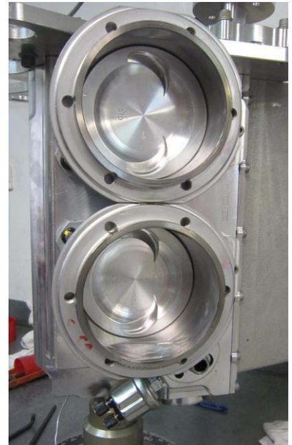
Figure 132 – Installation of Pistons With Valve Relief
