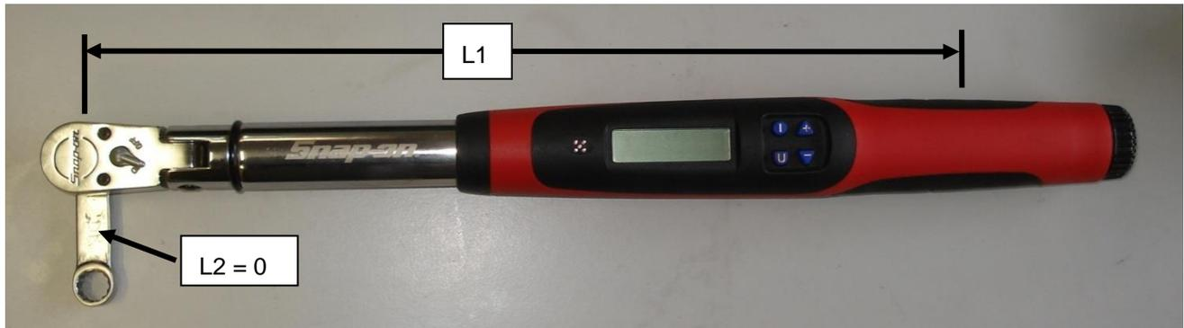
Figure 39 – Torque Wrench & Crowsfoot Adaptor Setting 2
