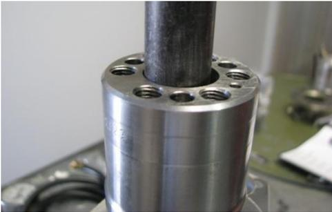
Essentially a long, large punch used to both remove and install the welch plugs from the ends of the crankshaft.
