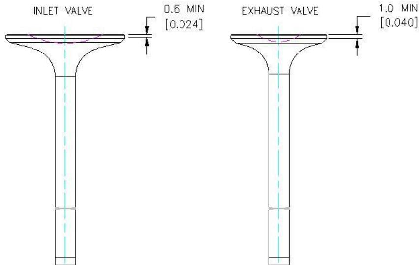
Figure 88 – Valve Measuring
