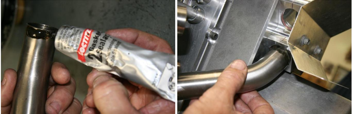
Figure 196 – Fitting Induction Pipes to Plenum Chamber
