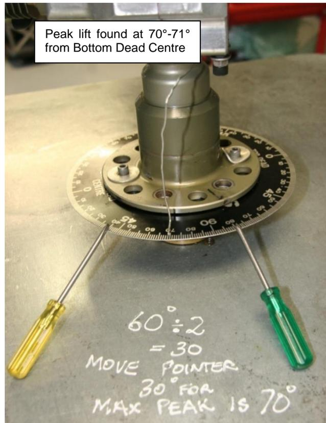
Figure 169 – Checking Cam Timing #2
