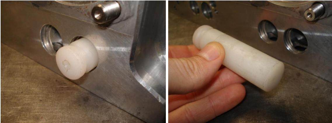
Figure 29 – Cam Timing Tool (Hydraulic Lifter)
