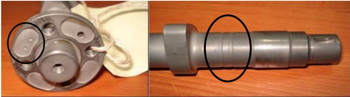
Figure 77 – 2-Ring Camshaft
