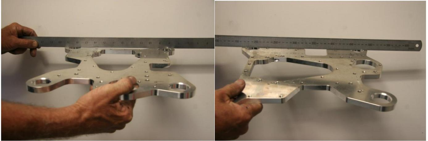
Figure 108 – Checking Engine Mount Plate Trueness
