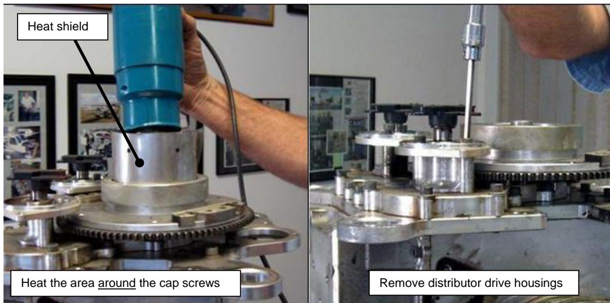
Figure 48 – Removing Flywheel Cap Screws & Distributor Drive Housings
