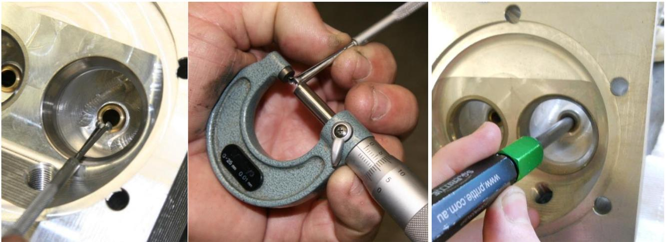
**Figure 91 – Measure Guide Wear (Telescopic Gauge Left & Middle, Go-No-Go Gauge Right)**
