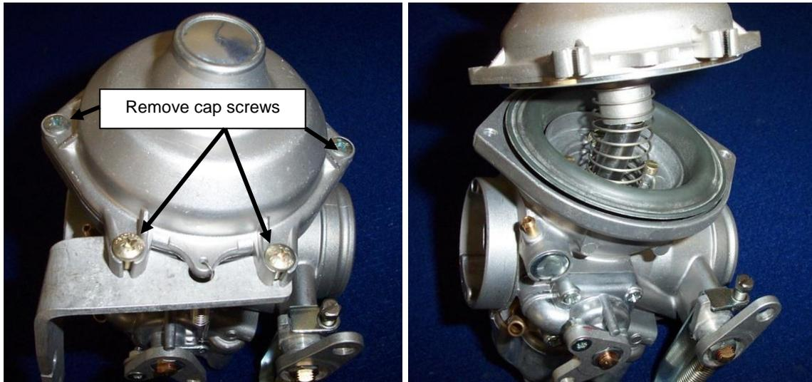
Figure 113 – Disassembling Carburettor #1
