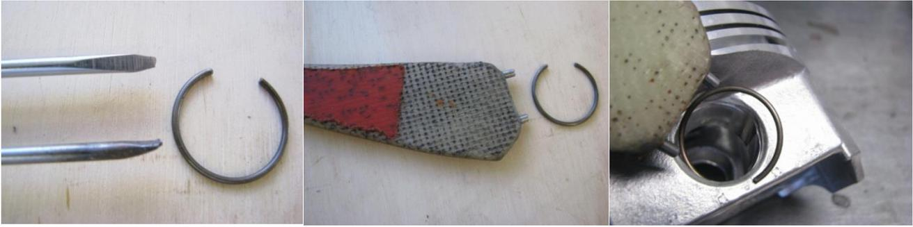
Figure 20 – Piston Circlip Remover and Installer
