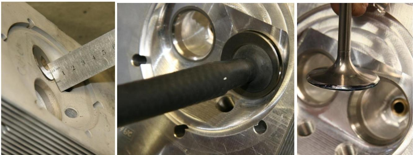
Figure 93 – Recessed Valve Seat, Valve Being Cut
