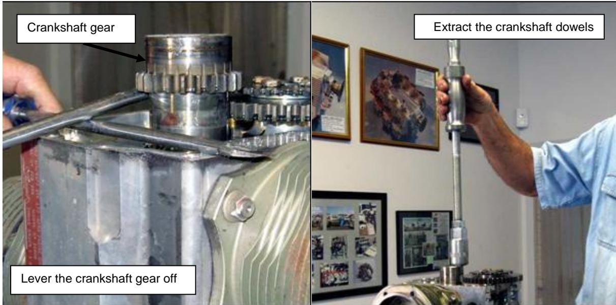
Figure 53 – Removing Crankshaft Timing Gear & Dowels
