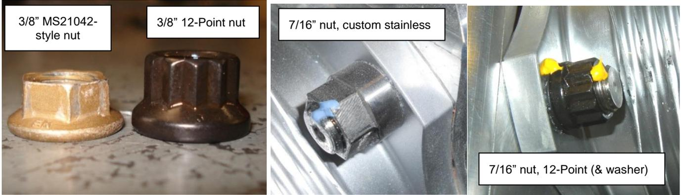
**Figure 143 – 12-Point Nuts, 7/16” Hardware (on right)**
