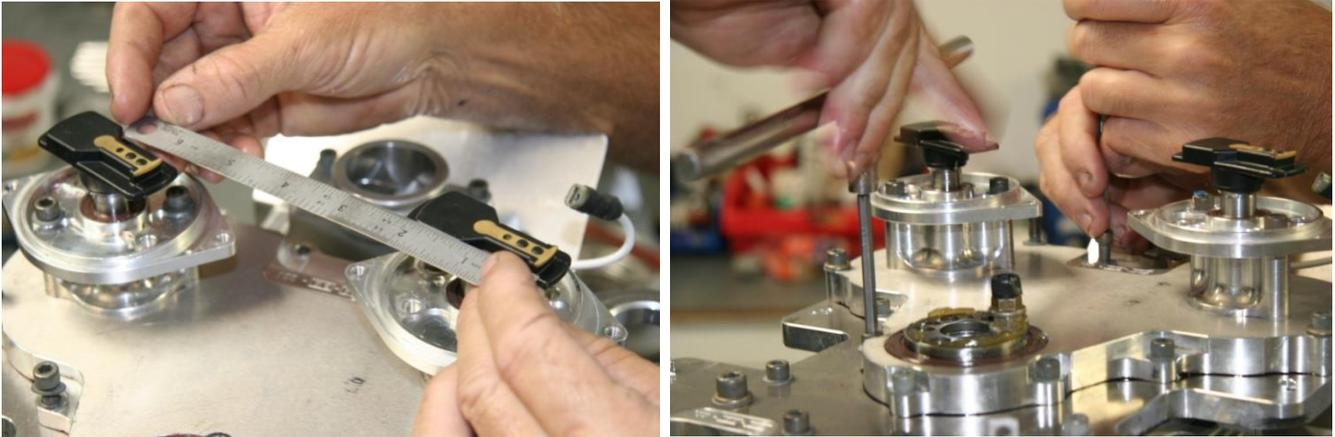
Figure 177 – Checking Rotors, Tightening Distributor Case
