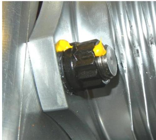
Figure 163 – Torque Seal Applied
