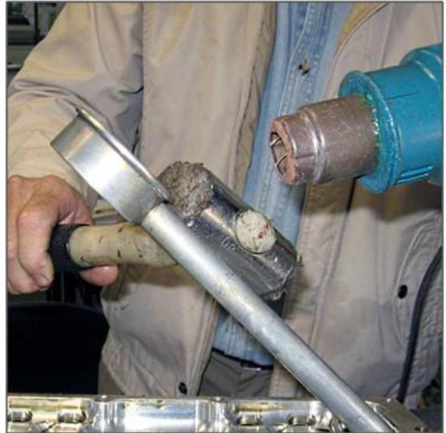
Figure 60 – Remove Oil Strainer
