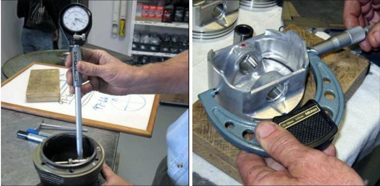
**Figure 85 – Measuring Cylinders & Pistons**
