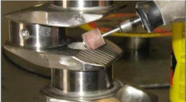
**Figure 67 – Radius Crank Centre Holes**
