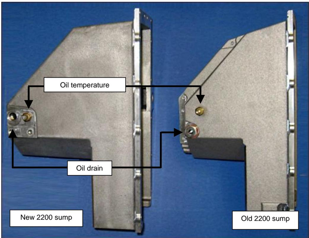
Figure 101 – 2200 Engine Sumps
