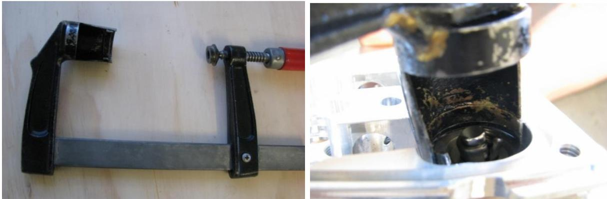
Figure 13 – Valve Spring Compressor / Collet Remover
