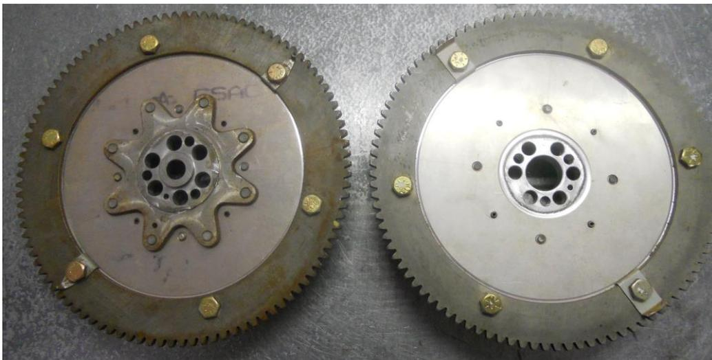
Figure 179 – Steel centred flywheel (left) aluminium flywheel (right).
