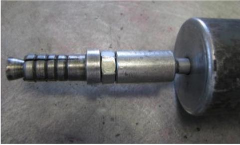
An adapted puller used to remove the dowel pins from the crankcase halves.
