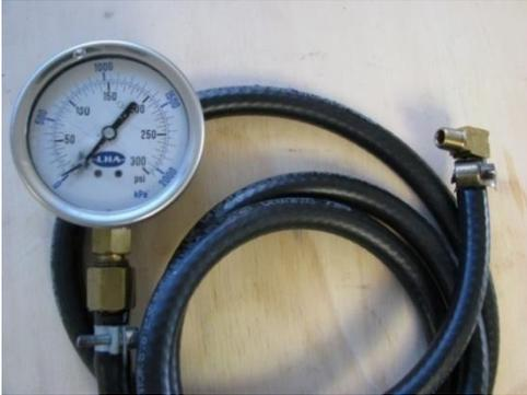
Used during initial engine proof runs and / or running-in. Used as a more accurate gauge to confirm the readings of the standard aircraft oil pressure gauge. Fitting uses 1/8 NPT thread.
