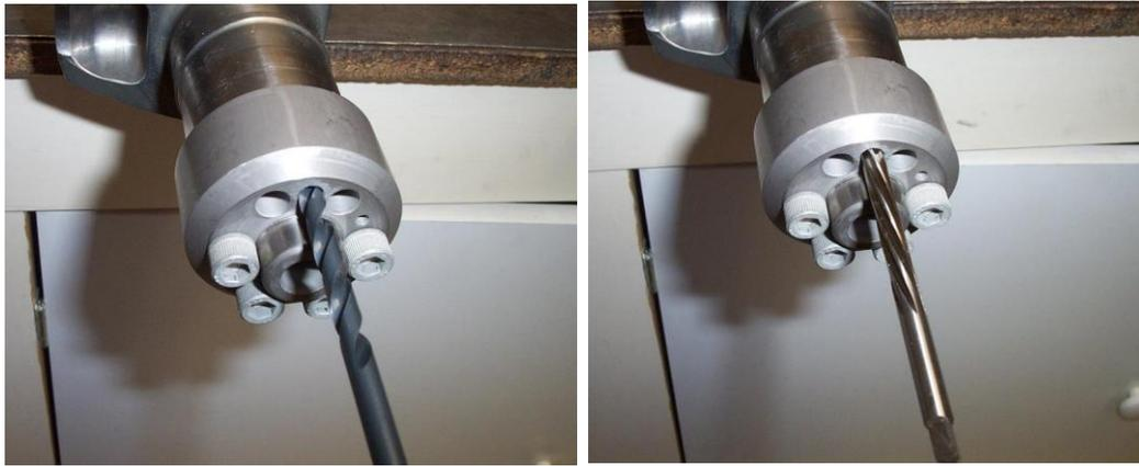
Figure 217 – Drilling & Reaming Crankshaft – ILLUSTRATION ONLY.
