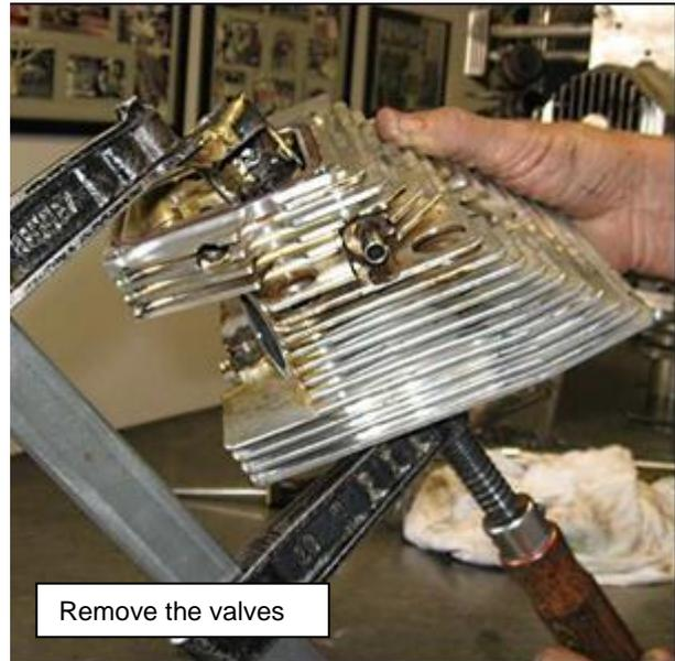
Figure 47 – Cylinder Head Disassembly
