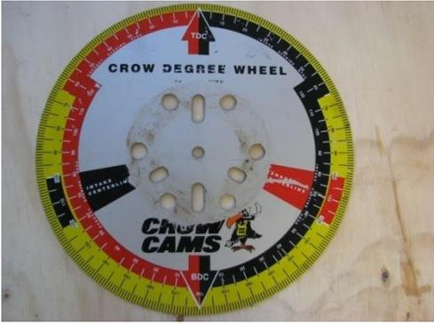
A degree wheel or degree disc – used during engine assembly to check engine timing.
