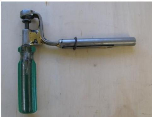
A screwdriver brazed to a modified spanner. Used to simplify adjusting the valve clearances in a solid-lifter engine. The spanner turns the rocker lock nut while the screwdriver turns the adjuster.
