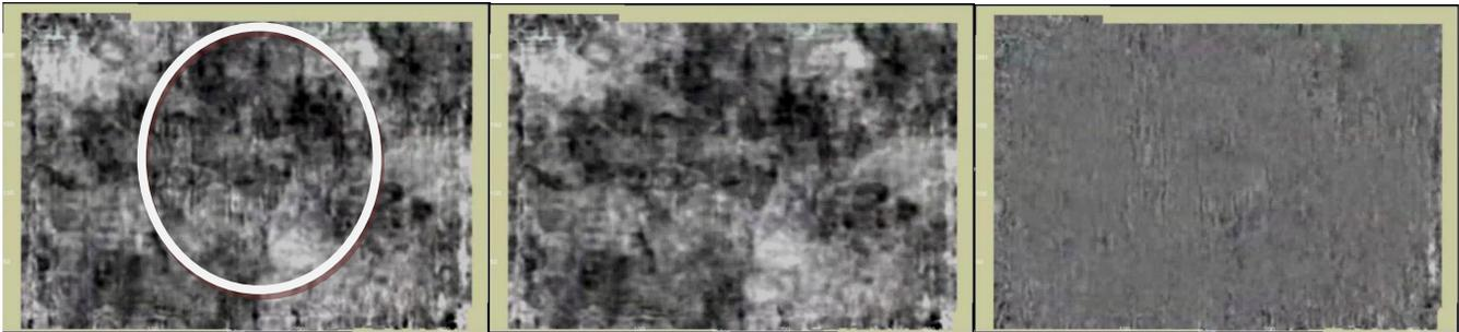
Figure 7: Left is the 5D only interpolated PSTM stack timeslice in the shallow, middle is the cascaded 2D and 5D interpolated PSTM stack timeslice and far right is the difference. The cascaded interpolated timeslice shows a clearer image with less vertical footprint/aliased noise as highlighted.
