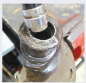
Continue to add more penetrating oil to the back side of the bushing for ease of removal.
