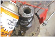
Next, you will need a bushing driver. Be sure to use a proper sized driver (kits can be purchased that contain multiple sizes) that engages the bushing edge but not the crankcase bushing hole. A 15/16" size worked in the picture to the right. Drive in the old bushing a short way to ensure a good fit.
