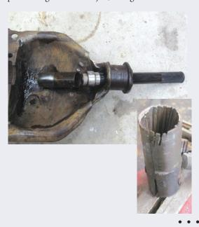
Now clean the bore of the hole and install the new crank handle bushing using the driver with a 2.5 pound mallet.
