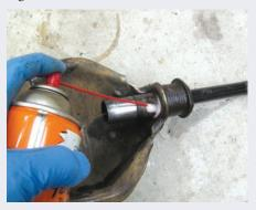
Continue driving the bushing until it is fully removed. With a very difficult bushing, you may have to use a hack-saw or metal cutting saw to make one or more cuts into the length of the bushing to allow it to collapse a bit. Most times the penetrating oil does the job, though.
