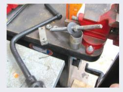
Alternately, a large threaded rod and assorted washers and sleeves can be used to pull or 'press' the bushing in place, as shown in the photo below.
