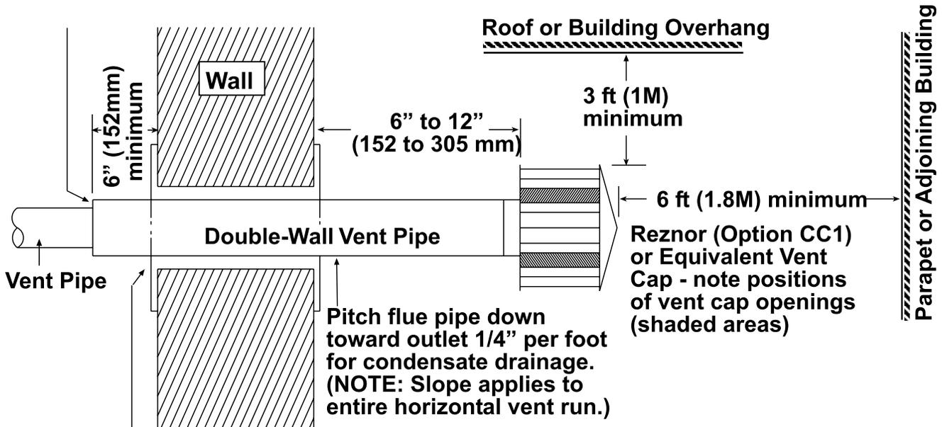
Approved clearance thimble is required when flue pipe extends through combustible materials. Follow the requirements of the thimble and/or the vent pipe manufacturer.
