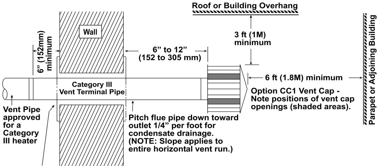
Approved clearance thimble is required when the flue pipe extends through combustible materials. Follow the requirements of the thimble and/or Category III vent pipe manufacturer.
