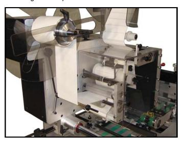
Run 3" wide labels on the standard KR 535. Even wider labels are possible using the optional 5" wide label kit.
