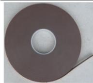
Doubled sided VHB tape is used to adhere new fence panel to existing railing. The same tape used to badge new vehicles.
