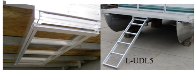
Five step extends 59" below the deck. Rated up to 300 lbs. Stows under the pontoon deck when not in use. Pulls out at an angle for easy boarding.
