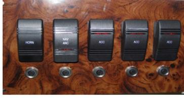
3 Standard switches, 1- 3 way switch for navigation & stern light, & 1- horn switch.
