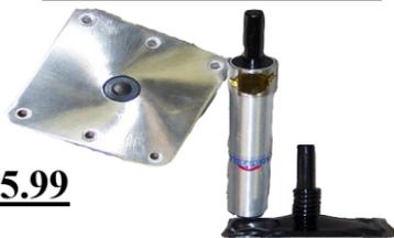
Floor plate, removable pin, & seat mount with spring. Use on fishing seats to move around the boat. **Extra floor plate \$28.95**
