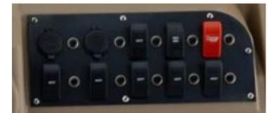
USB power outlets, 8 switches 5-10 amp & 3-5 amp breakers. Includes switch panel for right side and blank for left side of wheel on Premium Helm.
