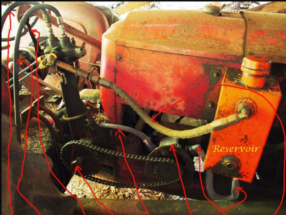
Up Down Actuator PTO Output Pump Suction Return
