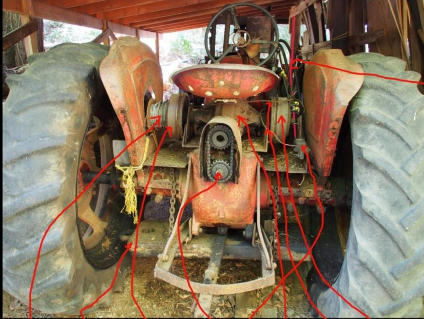
Cable Winch Braking Drum PTO Differential Driving Drum Elevator Weight Master Cylinder Brake Lines Operating Lever 1942 Massey Harris Row Crop Tractor With Continental Gas Engine With Rear PTO And Right Side PTO
