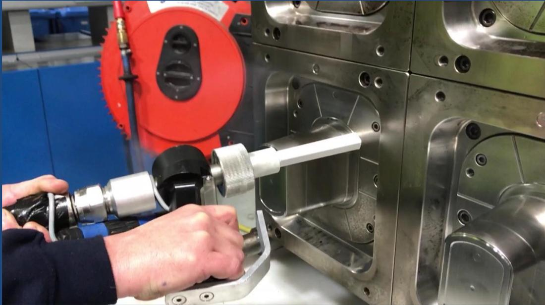
In situ on site cleaning without having to remove the moulds from the plastic injection moulding machine. Cleaning when hot is an advantage to the cleaning with dry ice. Quick return of equipment back into production. No need to cool down and reheat.
