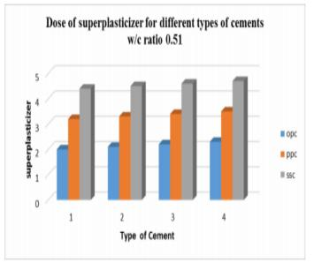
Fig.4: Dose of super plasticizer for different types of cements w/c ratio 0.51
