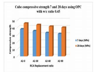
Fig.6: Cube compressive strength 7 and 28 days using OPC with w/c ratio 0.45
