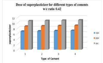
Fig.1: Dose of super plasticizer for different types of cements w/c ratio 0.42
