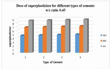
Fig.2: Dose of superplasticizer for different types of cements w/c ratio 0.45
