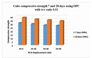
Fig.8: Cube compressive strength 7 and 28 days using OPC with w/c ratio 0.51
