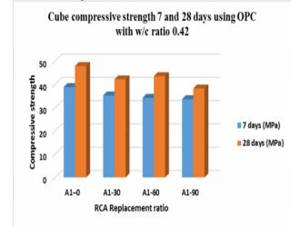
Fig.5: Cube compressive strength 7 and 28 days using OPC with w/c ratio 0.42
