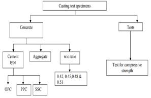
Fig.1: Experiment details for compressive strength
