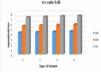
Fig.3: Dose of super plasticizer for different types of cements w/c ratio 0.48
