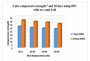
Fig.7: Cube compressive strength 7 and 28 days using OPC with w/c ratio 0.48
