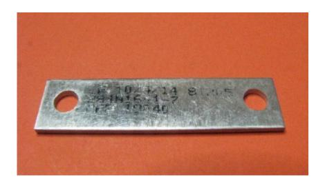
PMA Aeroparts announces the release of our latest FAA approved PMA product, Shim, P/N 284N1641-7AP. This product is an approved replacement for the OEM P/N 284N1641-7. This Shim is used on Boeing 737 Series 600, 700, 700C, 800, 900, and 900ER aircraft.
