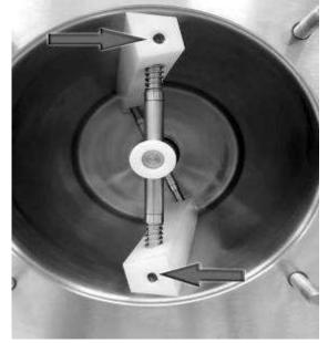
After the dasher is in place, you should be able to see the "dimple" on each of the two blades BEFORE you put the front door in place (see photo). If this is wrong the machine will not operate properly. You need to be aware of this Each and Every time you assemble the machine.
