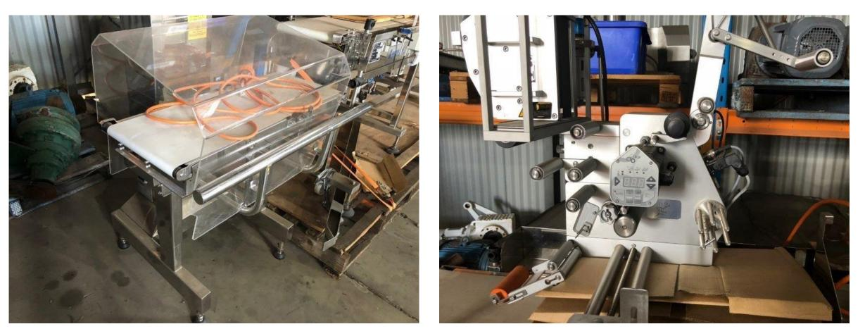
**Complete unit including check weigher / reject station/ labeller / printer/**
