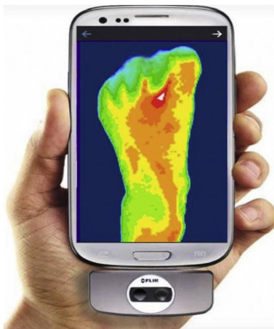
**Fig 1.** FLIR ONE thermal camera (FLIR Systems) is a smartphone-compatible device that captures thermal energy in the form of infrared radiation. The image shown in this smartphone is a left foot thermogram with normal tissue perfusion.
