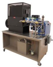
MODEL H-OBD-3 Mobile Dual-Fueled Burner Demonstrator Dimensions: 951/4"H x 60"W x 30"D (Shown without oil tank)
