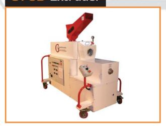
The G75D De-airing is a natural development of the well proven G75. The machines primary advantage over the G75 is that it uses a Duplex extruder construction and is fitted with a Vacuum chamber and high performance vacuum pump, this de-airs the modelling clay as it passes through the machine.
