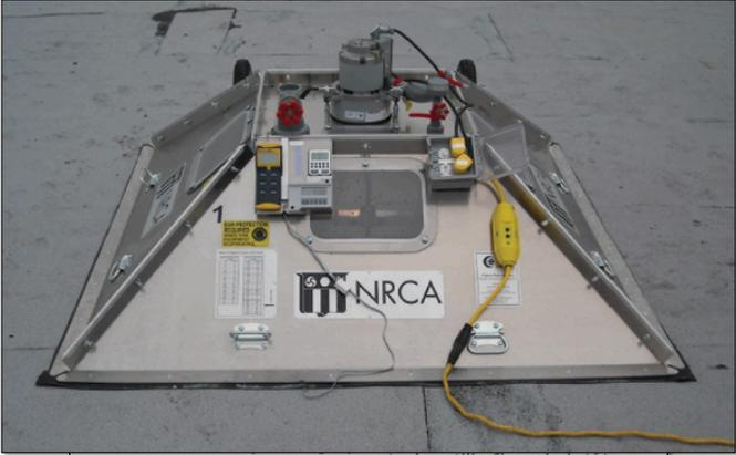
5-foot dome-like chamber to a roof surface's topside and applying a defined negative (uplift) pressure inside the chamber to the roof system's accessible surface using a vacuum pump (see photos). During the test, membrane surface deflection inside the chamber is visually monitored and measured to determine whether a roof system passes or is "suspect."
