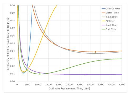
FIGURE 1 - COST PER UNIT TIME CURVES FOR EACH COMPONENT
