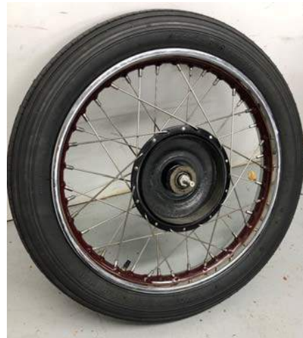
Turning the Brake Drum Can Be Done Without Dismantling the Wheel
