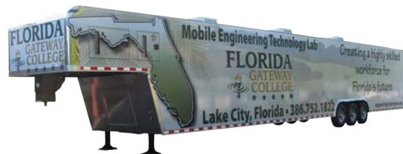
The 52' mobile classroom is set up as a training environment for 12-14 students at various stations. Trailer also includes two side mounted doors that raise up to allow for open classroom environment, as well as two side access doors and one large transportation door in back for movement of equipment.
