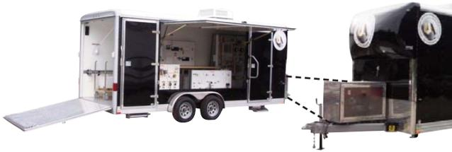
The 20' mobile classroom is set up as a training environment for 3-6 students at various stations. Trailer also includes one side mounted door that raises up to allow for open classroom environment, as well as two side access doors and one large transportation door in back for movement of equipment.
