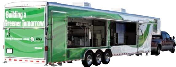
The 44' mobile classroom is set up as a training environment for 10-12 students at various stations. Trailer also includes two side mounted doors that raise up to allow for open classroom environment, as well as two side access doors and one large transportation door in back for movement of equipment.
