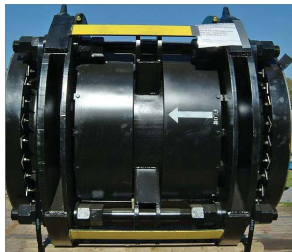
Ø36 inch diameter Universal expansion joint for a cycle gas service. Inco 600 redundant ply testable bellows with root rings. 422 psig at 302°F
