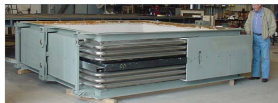
120 inch square hinged refractory lined universal expansion joint for a refinery. Inco 600 bellows with rounded corners. 2 psig at 1200°F
