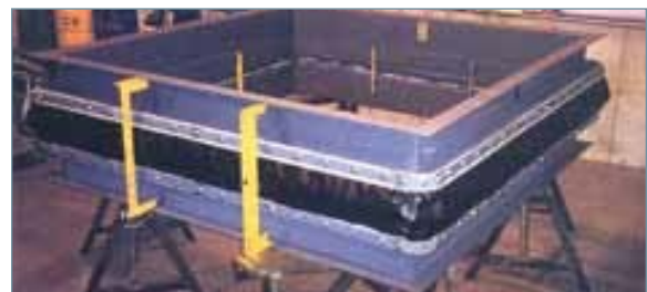
8 foot square boiler flue gas expansion joint. 20 in wc at 800°F
