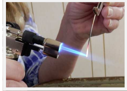
Using a torch to make a pinhead.
