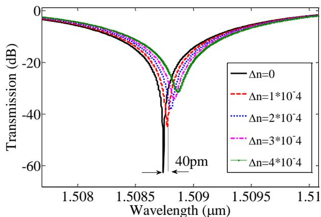
Figure. 5. Alternations of transmission with change effective index  $10^{-4}$
