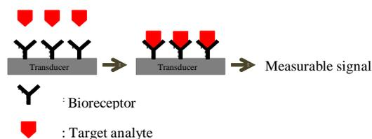
Figure 1. Schematic of a label-free biosensor
