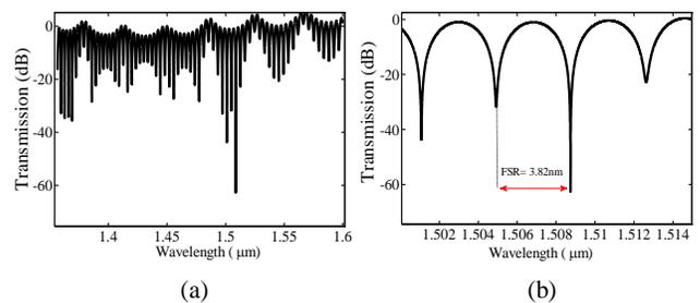
Figure 4. Sharp response and FSR are shown in fractal structure
