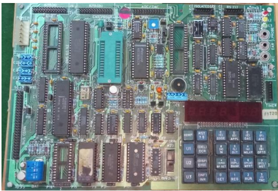
Fig.1: Microprocessor trainer kit with keypad and seven segment display
