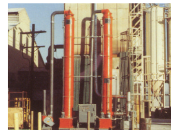
Special multi-stage gas scrubber field-tested unit
