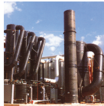
Multi-stage NO x , HCl, Cl 2 systems
