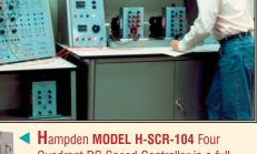
Quadrant DC Speed Controller is a fullwave regenerative drive capable of operating DC, PM or Shunt Motors in a bidirectional mode.
