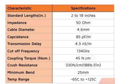
ConductRF 1.0mm Flexible VNA Test Cables are a proven solution for quality stable testing up to 110GHz. These cables have a minimum bend of 25mm(1.0"). Each assembly is serialized and supplied in a protective tube with test data.
