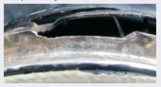
Use of a blunt tool or screwdriver tip can help to spin the reflector to clear the grooves. Some reflectors have a hole that can be used for turning.
