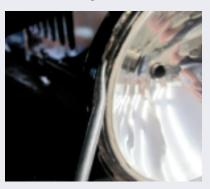
When replacing the reflector, be sure the 'fingers' on the spring in the bucket edge are pointing outward. Also, the cotton-cord gasket should be in place, with the end gap at the lower edge to help relieve moisture. Gasket cement will hold this cotton cord in place.
