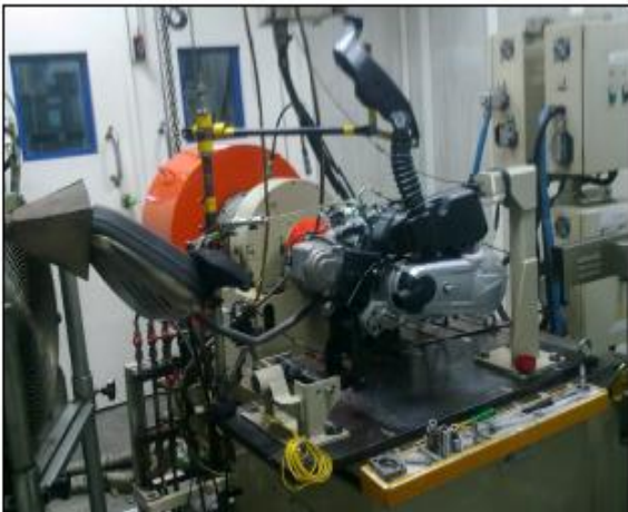
Fig.1: Vespa 125cc engine test rig
