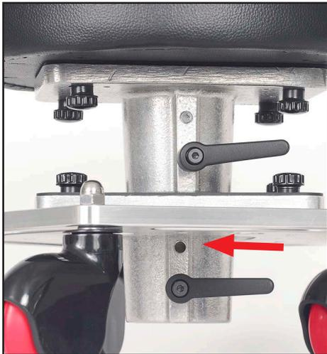
\* Note: It is necessary to temporarily remove the lower Kipp handle from the Base Flange in order for it to fit through the bottom of the Sneaker Base. (see red arrow) Only 1 Kipp handle is used in the Base Flange when installed inverted.
