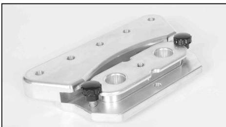
For storage, the support insert can be secured with two fastening knobs
