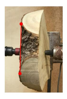
After checking the alignment, positon the two closest together high points so they are in vertical alignment when viewed from the tailstock.
