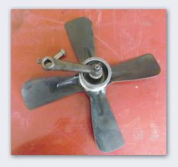
Remove the blade and pulley assembly from the fan bracket by first removing the cotter pin and shaft nut.
