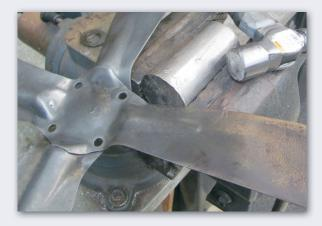
Assemble the cleaned and checked parts; add a touch of gasket cement to the gasket on the fan to pulley housing. Replace the fan blade screws and lock washers and tighten the fan to the pulley.
