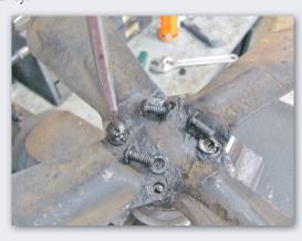
The pulley housing is now open and the end of the fan shaft is exposed. Since the shaft end has two flat areas on its edge, the appropriate tool is needed to turn the threaded shaft out of the threaded fan bracket. Holding the bracket in place and using a Crescent wrench on the fan shaft is one way to remove it.
