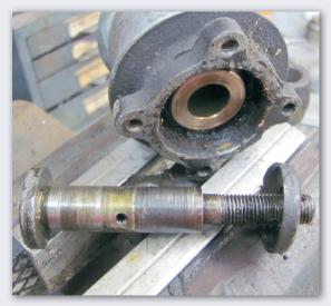
With the shaft removed, check wear of the bushing and replace the bushings and shaft with new ones as needed. Once the shaft and bushings are cleaned, checked, and free, oil the shaft and place it back into the cleaned pulley. Be sure the fan shaft internal oil passage is free. Sometimes grease is used in the fan hub and it can accumulate and plug the flow of lubricant; heavy oil is preferred.
