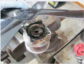
As the last step, add heavy weight oil (600 wt rear axle fluid may be used) to the pulley housing into the oil opening. Fill to the top of the opening and replace the oil plug. The fan assembly is now complete and ready to install on the car. Be sure to place a cotter pin in the large fan bracket bolt so the bolt won't turn loose and cause a rattling noise.
