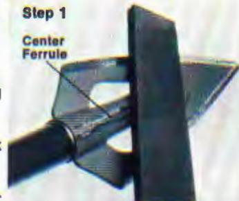
First filing, be sure to scratch up the center ferrule while you're filing the blade to make sure you're getting the correct angle of the blade.
