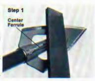
First filing, be sure to scratch up the center ferrule while you're filing the blade to make sure you're getting the correct angle of the blade.
