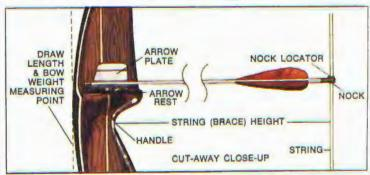
First method Draw a measuring arrow (marked in inches) in your bow. At full draw, your correct arrow length stops at the front of the arrow shelf
