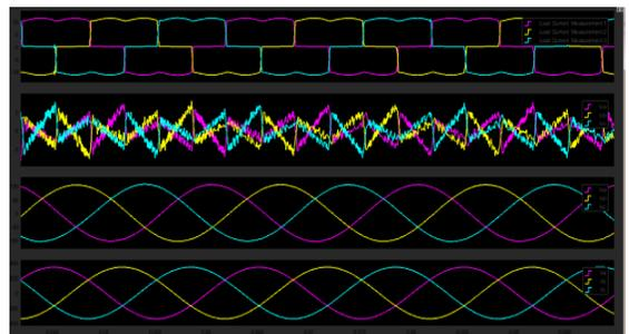
Fig.10: Waveforms of Load current, compensating current, supply current and supply voltage respectively (with SHPF)
