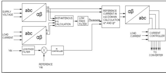
Fig.3: Control Algorithm p-q Theory
