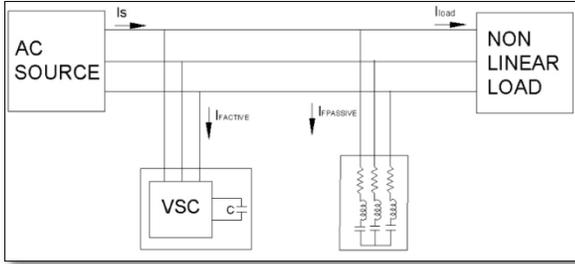
Fig.2: Block diagram of SHPF
