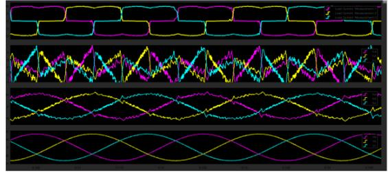
Fig.8: Waveforms of Load current, compensating current, supply current and supply voltage respectively (with SAPF)
