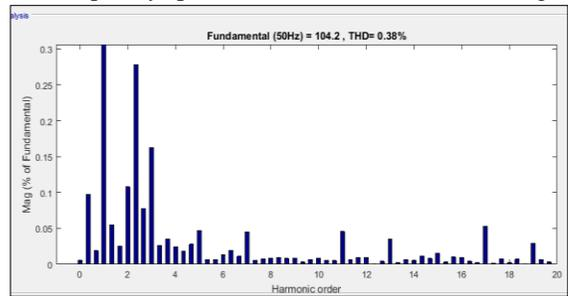
Fig.9: THD when Hybrid filter is connected
