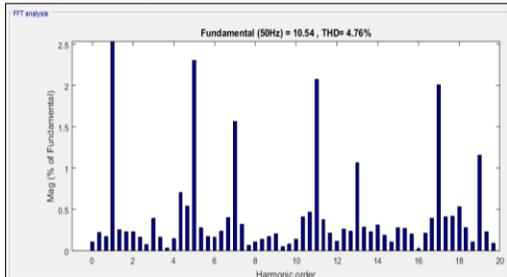
Fig.7: THD when active filter is connected
