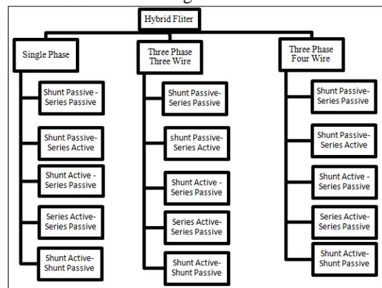
Fig.1: Hybrid Power Filter
