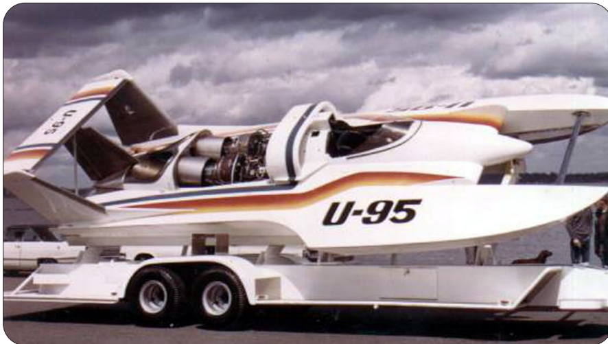
TOP: The arrival of the U-95 to the Stan Sayres Pits in Seattle in 1973 caused quite a sensation among the hydro fans. Here, the crowd stands there gawking at the strange thing. MIDDLE: Leif Borgersen in the cockpit of the U-95. ABOVE: The U-95 as it was painted for the 1974 season and with its twin Lycoming T53-L-13 gas turbine engines on display.
