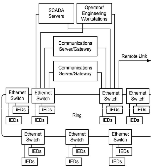
Fig. 11. Typical substation network with ring architecture
