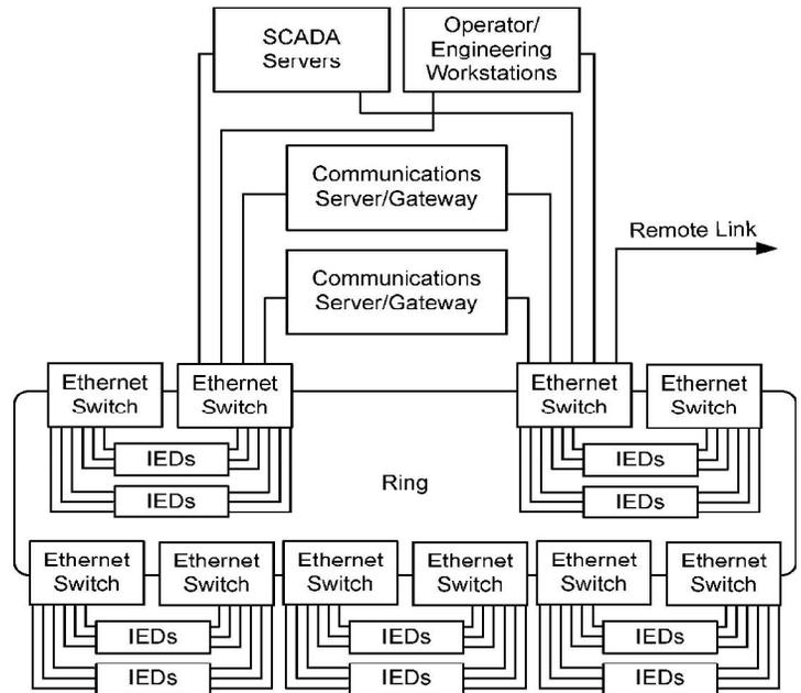
Fig. 12. Typical substation network with ring architecture and dual-port IEDs
