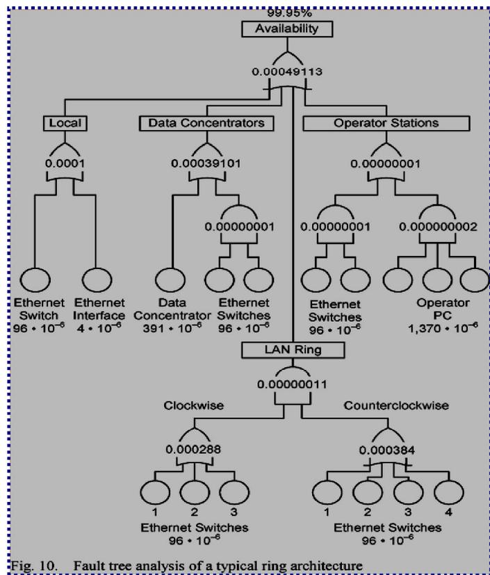
Fig. 10. Fault tree analysis of a typical ring architecture
