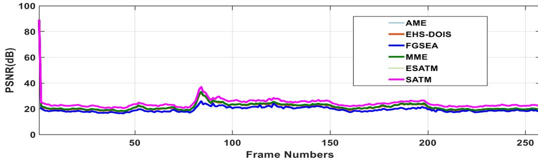
Figure 5: The average PSNR(dB) in each frame for various algorithms using foot ball video sequence.
