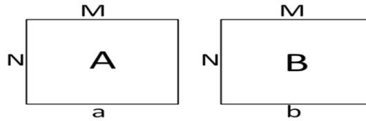
Figure 1: (a) Macro block (b) Candidate block of size M X N respectively.
