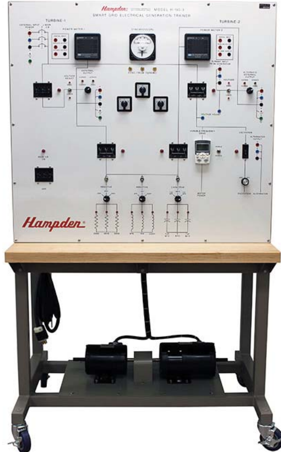
Hampden Model H-190-3 Electrical Generation Synchronization Trainer Dimensions: 75"H x 44"W x 32"D Shipping Weight: 854 lbs.
