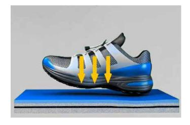
The area of deformation on point-elastic flooring is much smaller than area-elastic systems; the surrounding areas of the floor remain relatively unchanged by activity in a particular area.
