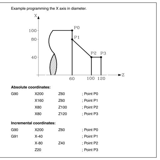
On power-up, after executing M02, M30 or after an EMERGENCY or RESET, the CNC will assume G90 or G91 according to the definition by the general machine parameter "ISYSTEM".
