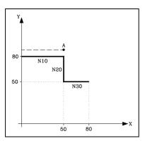
Block N15 interrupts block preparation and the execution of block N10 will finish at point A.
