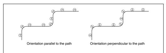
The path is defined by the axes of the active plane. The axis maintaining the orientation must be a rotary rollover axis (A, B or C).
