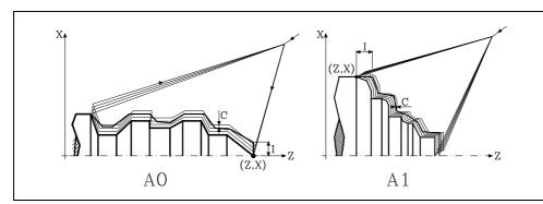
When not programming the A parameter, the "I" and "C" values depend on the tool dimensions..
