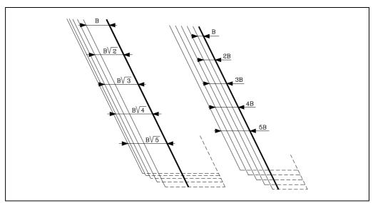
• If a positive value is programmed, the depth of each pass will depend on the number of the corresponding pass.
