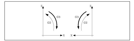
Circular interpolation can only be executed on a plane. The form of definition of circular interpolation is as follows :
