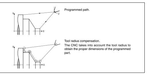
The CNC does not show the tool center path; it shows the position of the theoretical tip.
