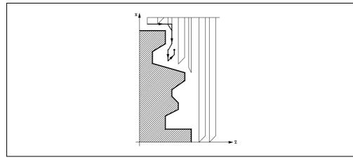
To do this, it will return in G00 to the point where the machining of the profile was interrupted.
