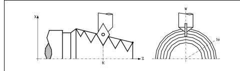
• If parameter "K" has not been defined, it indicates the angular position of the spindle corresponding to the thread's starting point. This allows making multi-entry threads without using the parameter "V".
