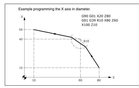
PATH CONTROL Chamfer (G39)
