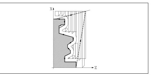
Once the finishing pass has ended, the tool will return to the point from where the cycle was called.
