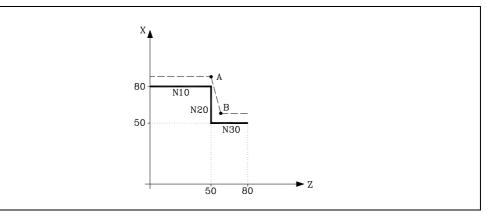
As you can see, the resulting path is not the required one, so we recommend avoiding the use of function G04 in sections which work with compensation.
