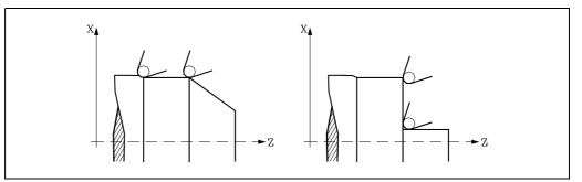
There are problems in incline sections (left figure) and on rounded sides (right figure).
