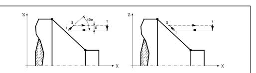
When programming D with a value other than 0, the cutter withdraws at 45<sup>o</sup> until reaching the safety distance (left figure).
