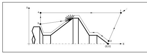
4. The canned cycle will always end at the point where the cycle was called from.
