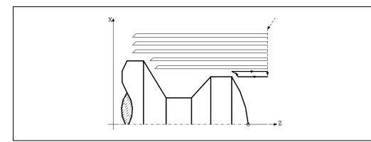
Once the CNC is done machining the excess profile, it will start executing the detected channels.
