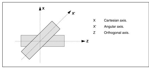
Programming in the Cartesian system (Z-X) requires activating an angular transformation of an inclined plane that converts the movements of the real (non-perpendicular) axes (Z-X'). This way, a movement programmed on the X axis is transformed into movements on the Z-X' axes; i.e. it then moves along the Z axis and the angular X' axis.
