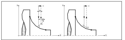
It must be borne in mind that when not programming the parameter D, the cycle execution time is greater but the finishing stock is smaller.
