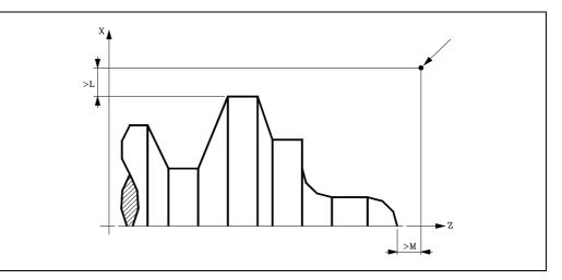
If the tool position is not correct to execute the cycle, the CNC will display the corresponding error.
