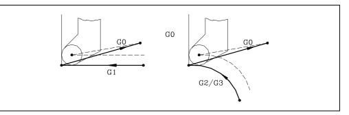
When detecting a change from G00 to G01, G02, G03, G33 or G34, the new block is treated like the first compensated point resuming tool radius compensation.
