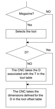
If the machine has a tool magazine, the CNC looks up the "Tool magazine table" to know the position occupied by the selected tool and the desired one.
