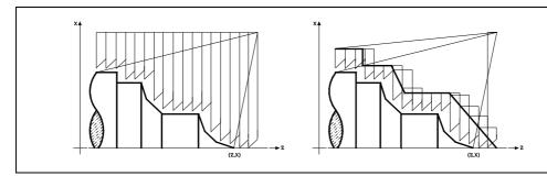
When the stock profile is known, it is recommended to define both profiles: The profile of the original stock and the desired final profile. The machining operation is much faster because only the stock delimited by both profiles is removed.
