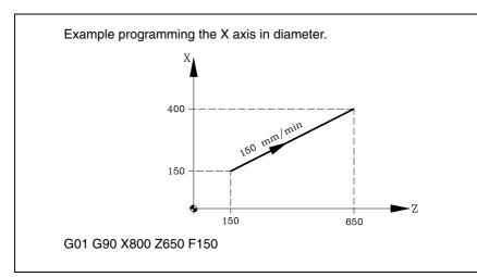
The programmed feedrate "F" may vary between 0% and 120% via the switch located on the Control Panel of the CNC, or by selecting between 0% and 255% from the PLC, or via the DNC or the program.
