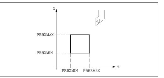
To execute the cycle, a master tool of known dimensions will be used with its relevant values previously entered in the selected offset. Since the probe needs to be calibrated along the X and Z axes, the location code (F) of the selected master tool must be F1, F3, F5 or F7.
