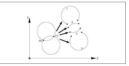
If P0 is the starting point and P1 the endpoint, there are 4 arcs which have the same value passing through both points.
