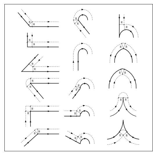
The way the various paths are blended (joined) depends on the setting of machine parameter COMPMODE.
