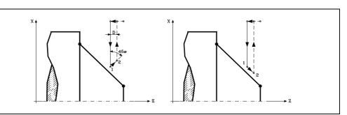
When programming D with a value other than 0, the cutter withdraws at 45<sup>o</sup> until reaching the safety distance (left figure).
