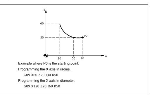
Function G09 is not modal, so it should always be programmed if you wish to execute an arc defined by three points. Function G09 can be programmed as G9.
