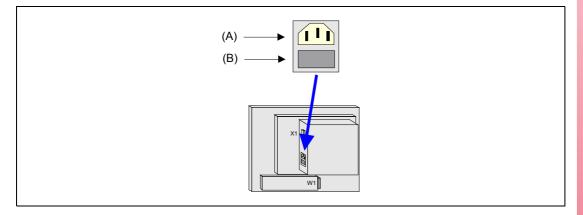
Before turning on the monitor of the 8055 CNC and verifying that the external AC line (B) fuse of each unit is the right one. See identification label of the unit itself.
