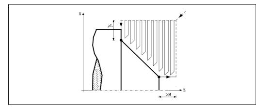
If the tool position is not correct to execute the cycle, the CNC will display the corresponding error.
