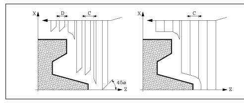
When programming D with a value other than 0, the cutter withdraws at 45<sup>o</sup> until reaching the safety distance (left figure).
