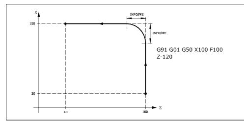
Function G50 assures that the difference between the theoretical and actual paths stays smaller than what was set by machine parameter "INPOSW2".
