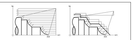
When the stock profile is known, it is recommended to define both profiles: The profile of the original stock and the desired final profile. The machining operation is much faster because only the stock delimited by both profiles is removed.
