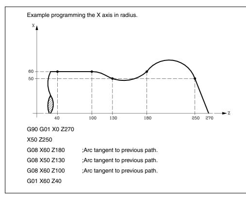
Function G08 is not modal, so it should always be programmed if you wish to execute an arc tangential to the previous path. Function G08 can be programmed as G8.
