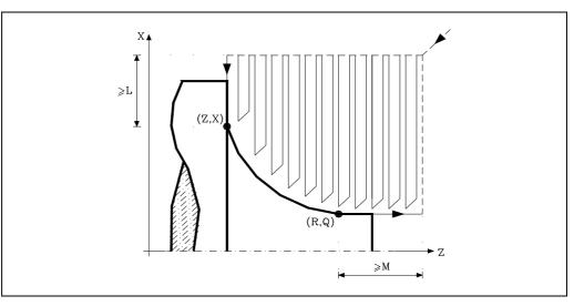
If the tool position is not correct to execute the cycle, the CNC will display the corresponding error.
