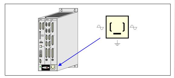
To prevent electrical shock at the monitor of the 8055 CNC, use the proper mains AC connector (A) with 3-wire power cables (one of them for ground connection).
