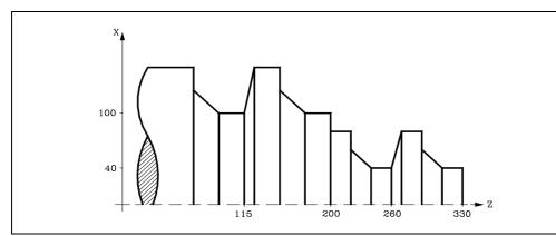
G90 G01 X80 Z330 (PCALL 10, P0=20, P1=-10) ; Also (PCALL 10, A20, B-10) G90 G01 X80 Z260 (PCALL 10, P0=20, P1=-10) ; Also (PCALL 10, A20, B-10) G90 G01 X200 Z200 (PCALL 10, P0=30, P1=-15) ; Also (PCALL 10, A30, B-15) G90 G01 X200 Z115 (PCALL 10, P0=30, P1=-15) ; Also (PCALL 10, A30, B-15) M30 (SUB 10) G91 G01 ZP1 XP0 ZP1 XP0 ZP1
