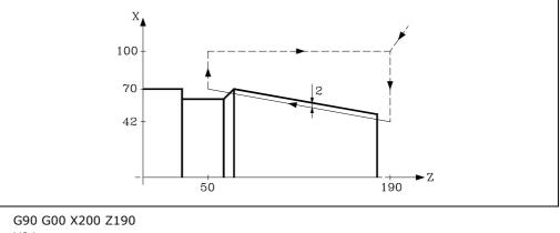
G90 G00 X200 Z190 X84 G33 X140 Z50 L5 ; First threadcutting. G00 X200 Z190
