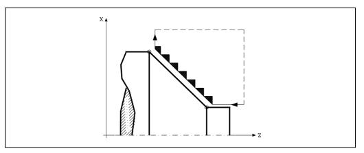
After the turning operation (with or without finishing pass) the canned cycle will always end at the cycle calling point.
