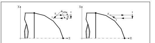
It must be borne in mind that when not programming the parameter D, the cycle execution time is greater but the finishing stock is smaller.
