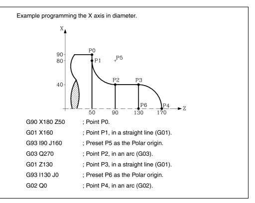
If G93 is only programmed in a block, the point where the machine is at that moment becomes the polar origin.
