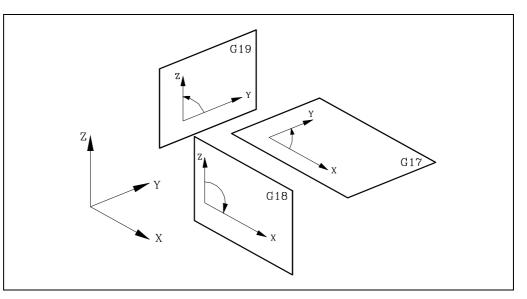
On power-up, after executing M02, M30 or after EMERGENCY or RESET, the CNC will assume that the plane defined by the general machine parameter as "IPLANE" is the work plane.
