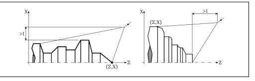
If the tool position is not correct to execute the cycle, the CNC will display the corresponding error.
