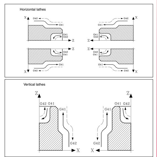
Tool COMPENSATION Tool radius compensation
