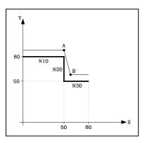
As the next point corresponding to the compensated path is point "B", the CNC will move the tool to this point, executing path "A-B".
