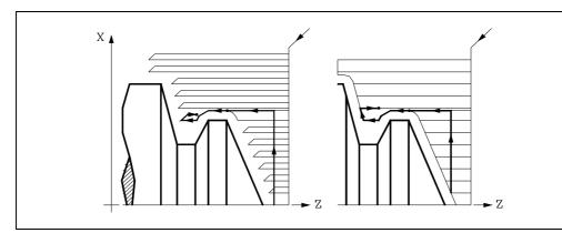
To do this, it will return in G00 to the point where the machining of the profile was interrupted.
