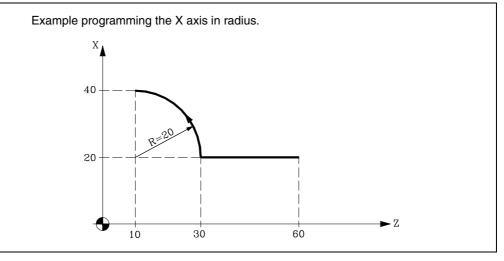
If the starting point is X20 Z60 and you wish to machine an arc (the path of approach being straight) you should program:
