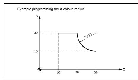
If the starting point is X0 Y30 and you wish to machine an arc (the exit paths being straight) you must program:
