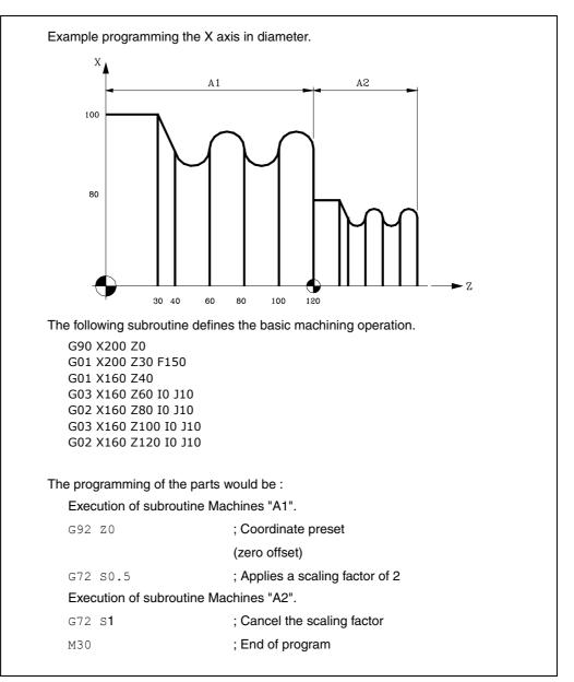
Function G72 is modal and is cancelled when another scaling factor with a value of S1 is programmed, or on power-up, after executing M02, M30 or after EMERGENCY or RESET.
