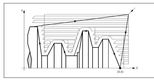
Once the finishing pass has ended, the tool will return to the point from where the cycle was called.
