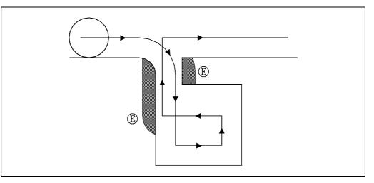
When detecting a loop or a collision, the blocks that caused it will not be executed and a warning will be issued for each loop or collision eliminated.
