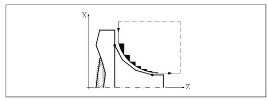
After the facing operation (with or without finishing pass) the canned cycle will always end at the cycle calling point.
