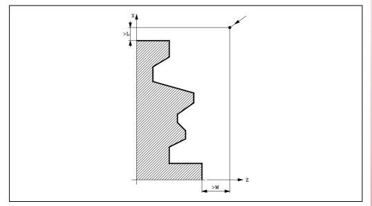
If the tool position is not correct to execute the cycle, the CNC will display the corresponding error.
