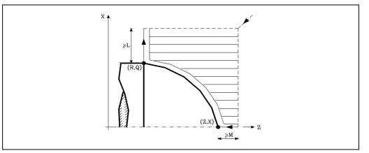
If the tool position is not correct to execute the cycle, the CNC will display the corresponding error.
