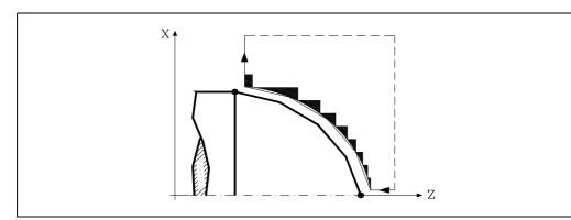
After the turning operation (with or without finishing pass) the canned cycle will always end at the cycle calling point.
