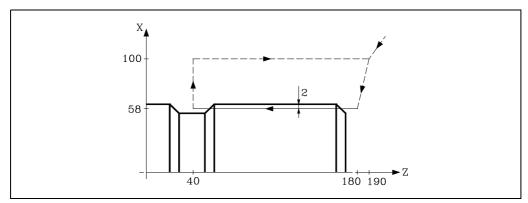
G90 G00 X200 Z190 X116 Z180 G33 Z40 L5 Q0 ; First threadcutting. G00 X200 Z190 X116 Z180 G33 Z40 L5 Q180 ; Second threadcutting. G00 X200 Z190
