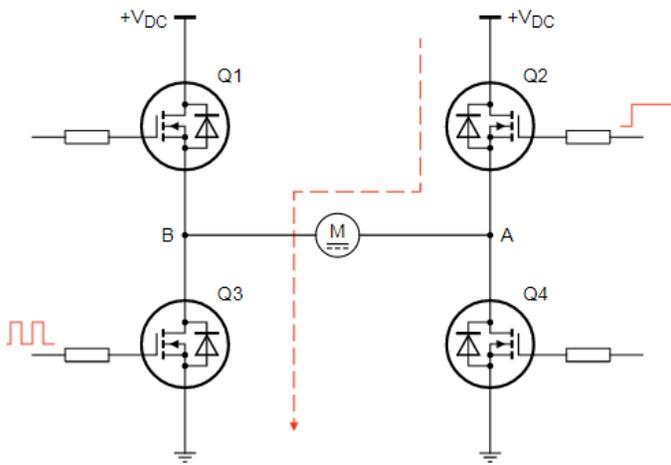
Figure 6: Unipolar drive H-bridge switching
