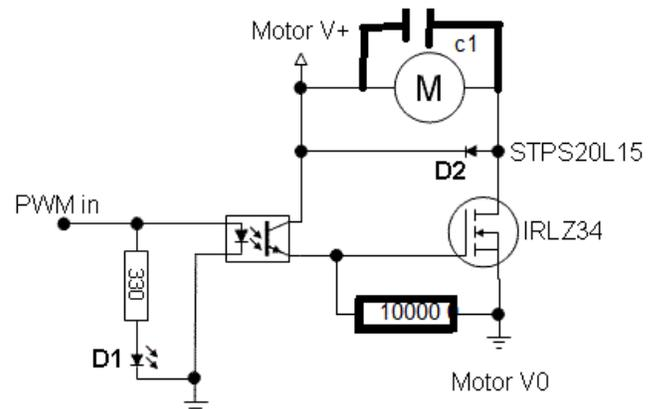
Figure 4: Circuit for Speed Control Using MOSFET
