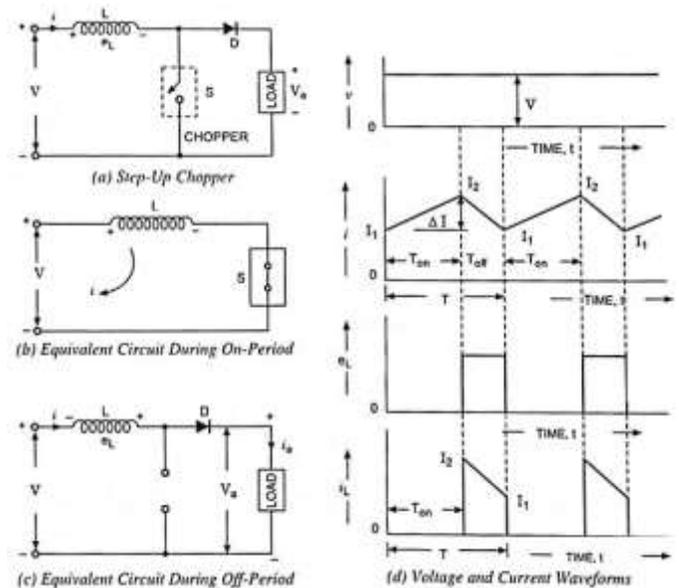
Figure 1: Basic Chopper circuit and its Waveforms
