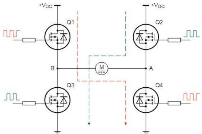
Figure 5: Bipolar drive H-bridge switching
