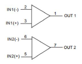
The Op-Amp here works as a Differential amplifier, where the output voltage is simply the difference between the two input voltages.
