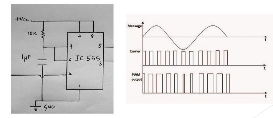
Here it serves the purpose of a Pulse Width Modulator.
