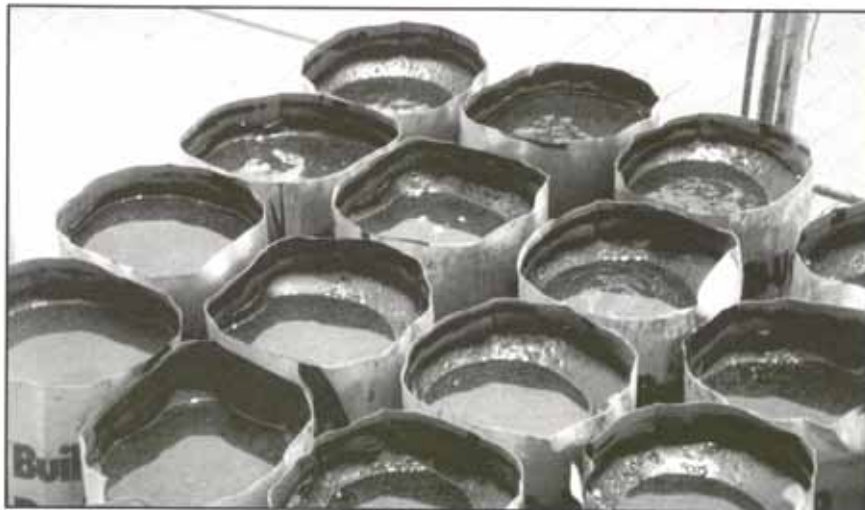
Water collecting on top of asphalt kegs.
