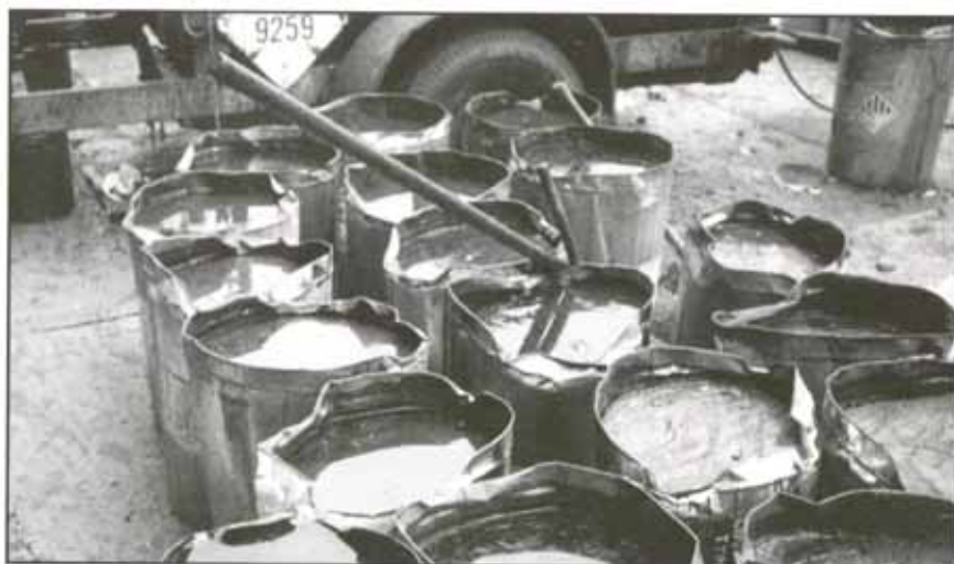
Water collecting on top of coal-tar pitch containers.
