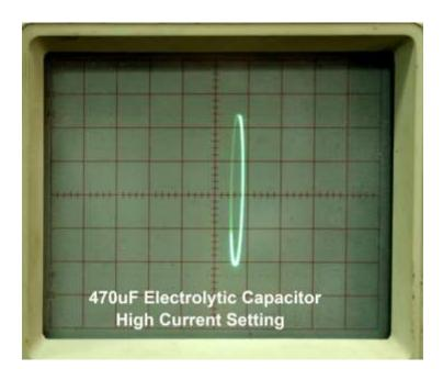
At times the oscilloscope controls may need altering to get the desired pattern shape and size, but often use of the High Low switch will negate this need to alter the 'scope settings.
